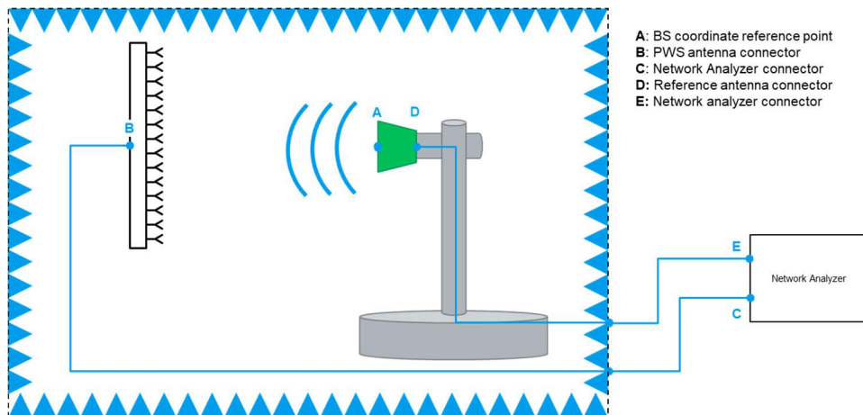
Figure 8.6-1: Path loss calibration in PWS, TX requirements
