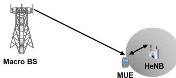
Figure 6.2.2.1-1 Assumed interference scenario for coexistence with uncoordinated UE
