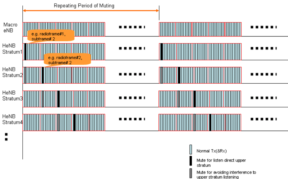
Fig. 6.4.2.1.4.2-1 Explanation for blind detection on stratum info and synchronization status
