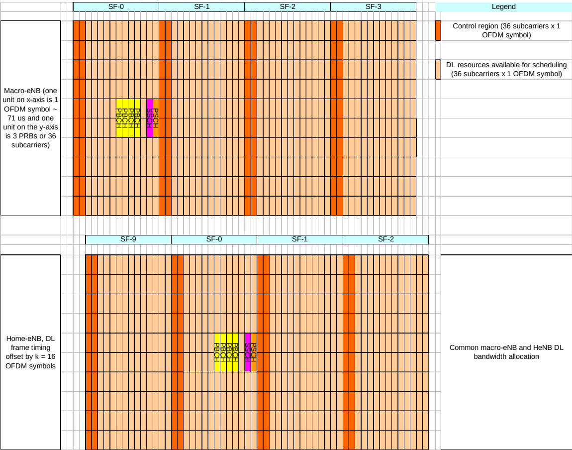
Figure 7.2.1.1 Time-shift HeNB frame timing by k = 16 OFDM symbols relative to macro-eNB timing
