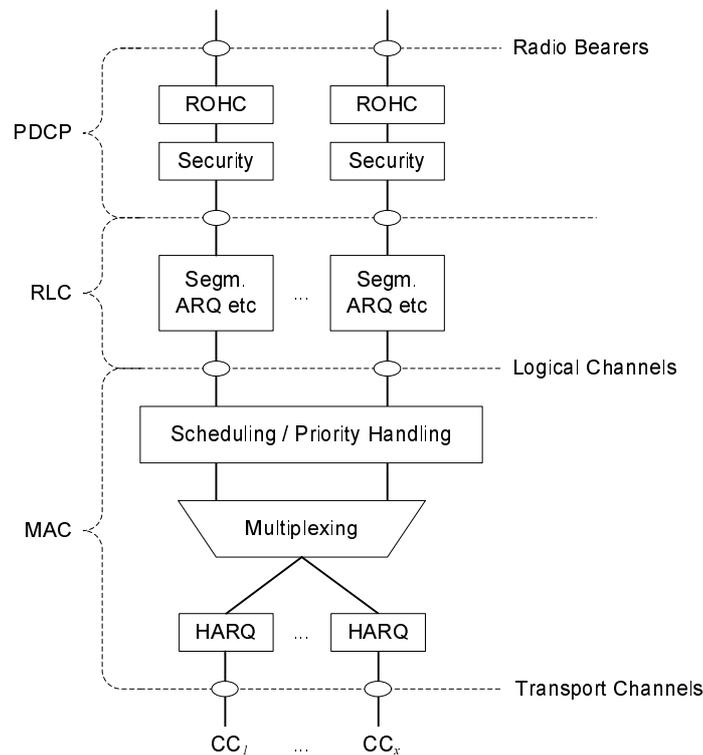
Figure 5.2.1-2: Layer 2 Structure for the UL
