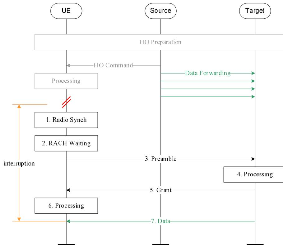
**Figure 16.5-1: U-Plane interruption in LTE-Advanced**
