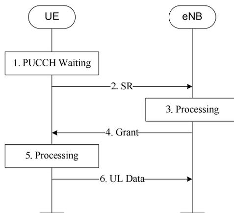
**Figure 16.2.2-1: Dormant to Active transition for synchronised UE**
