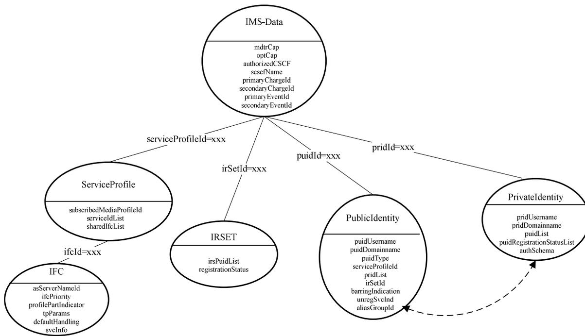
Figure 11.2.1-1: DIT Structure for IMS-Data with Alternative A
