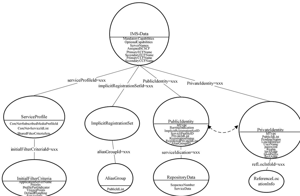
Figure 11.2.2-1: DIT Structure for IMS-Data with Alternative B
