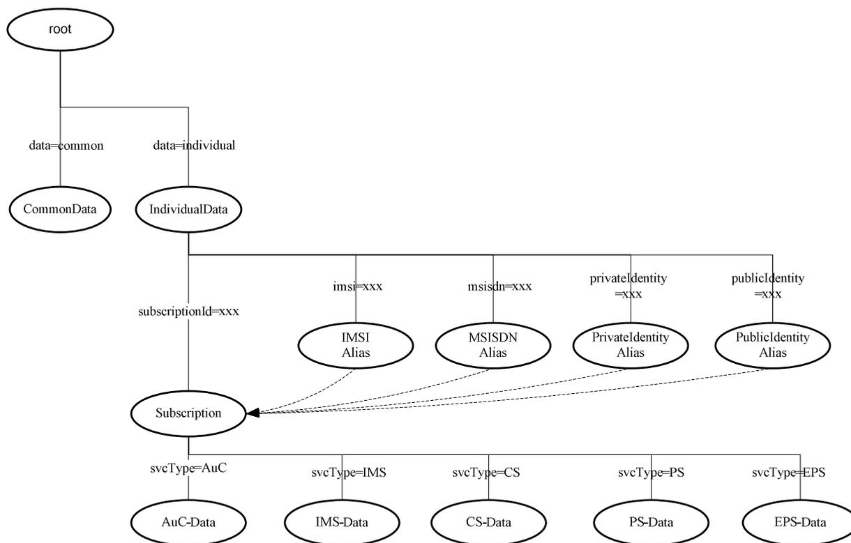
**Figure 6.2.2-1: DIT Structure for UDC with alternative B**
