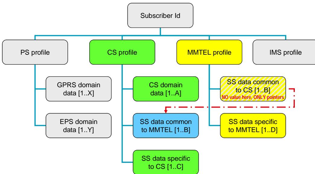
Figure 4.2.5-2: Reference Data Model referring to CS services
