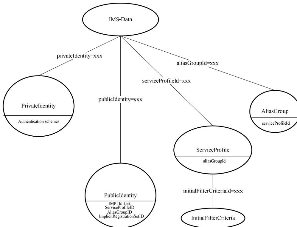
Figure 11.2.4-1: DIT Structure for IMS-Data with Alternative D
