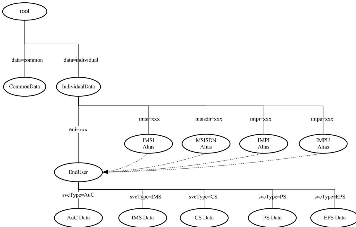
**Figure 6.2.1-1: DIT Structure for UDC with alternative A**
