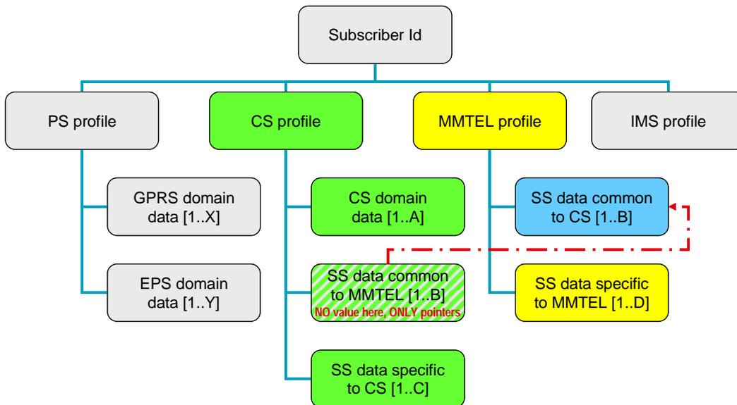
Figure 4.2.5-1: Reference Data Model referring to MMTEL services
