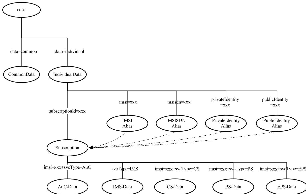
Figure 6.2.4-1: DIT Structure for UDC with alternative D
