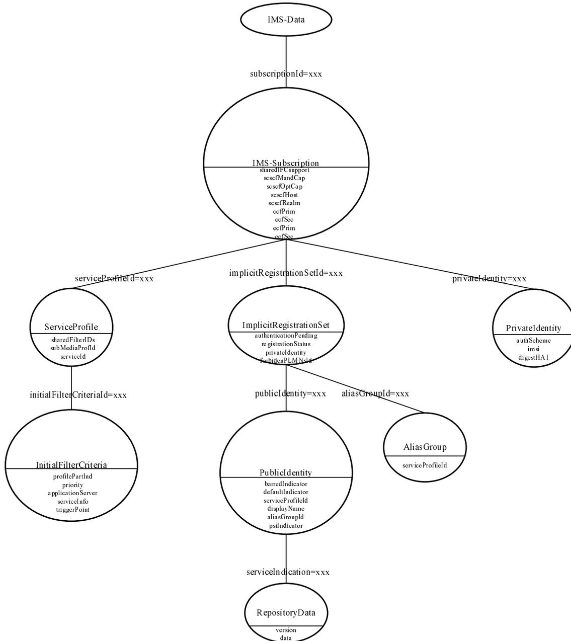
Figure 11.2.3-1: DIT Structure for IMS-Data with Alternative C
