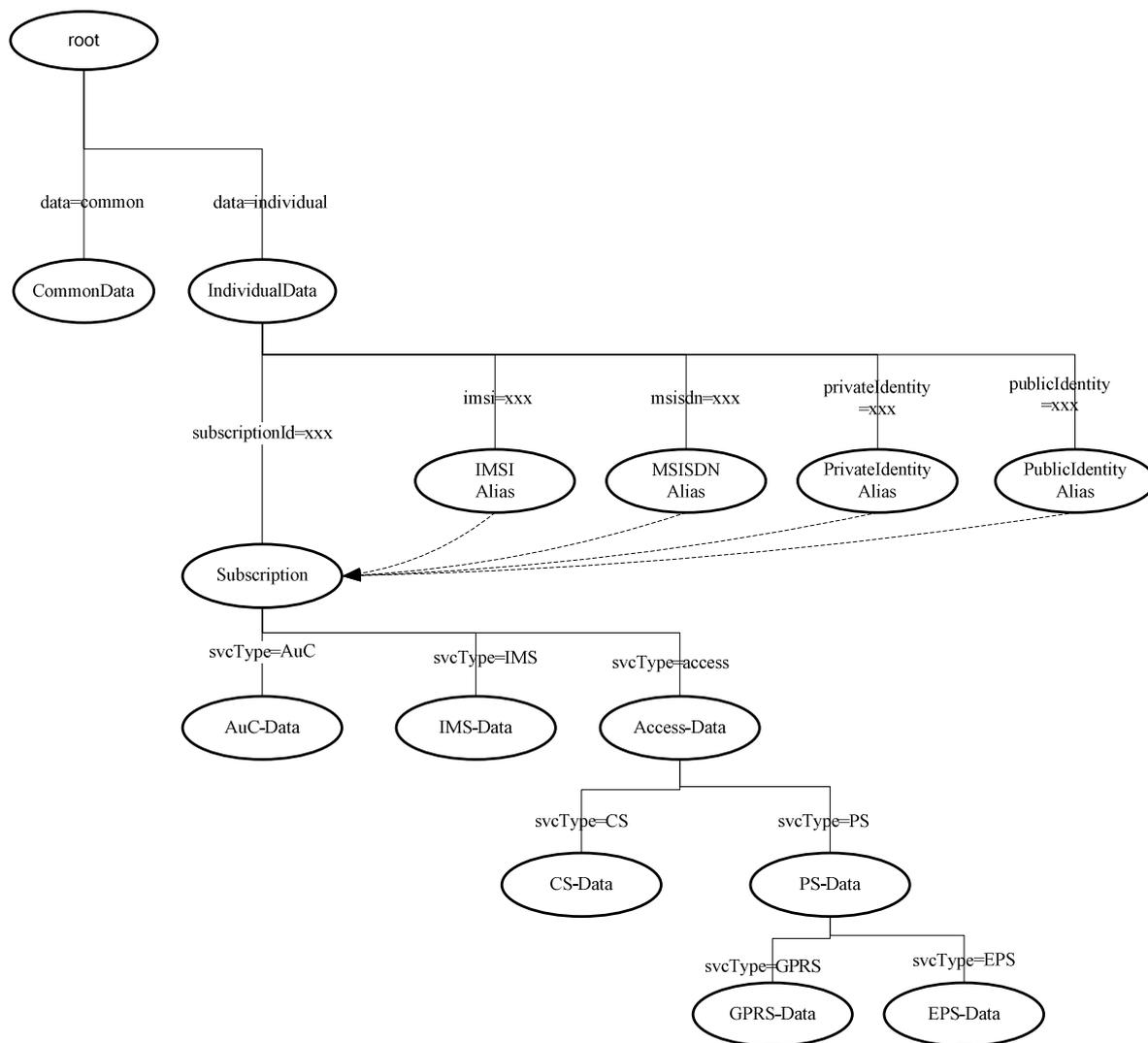
Figure 6.2.3-1: DIT Structure for UDC with alternative C
