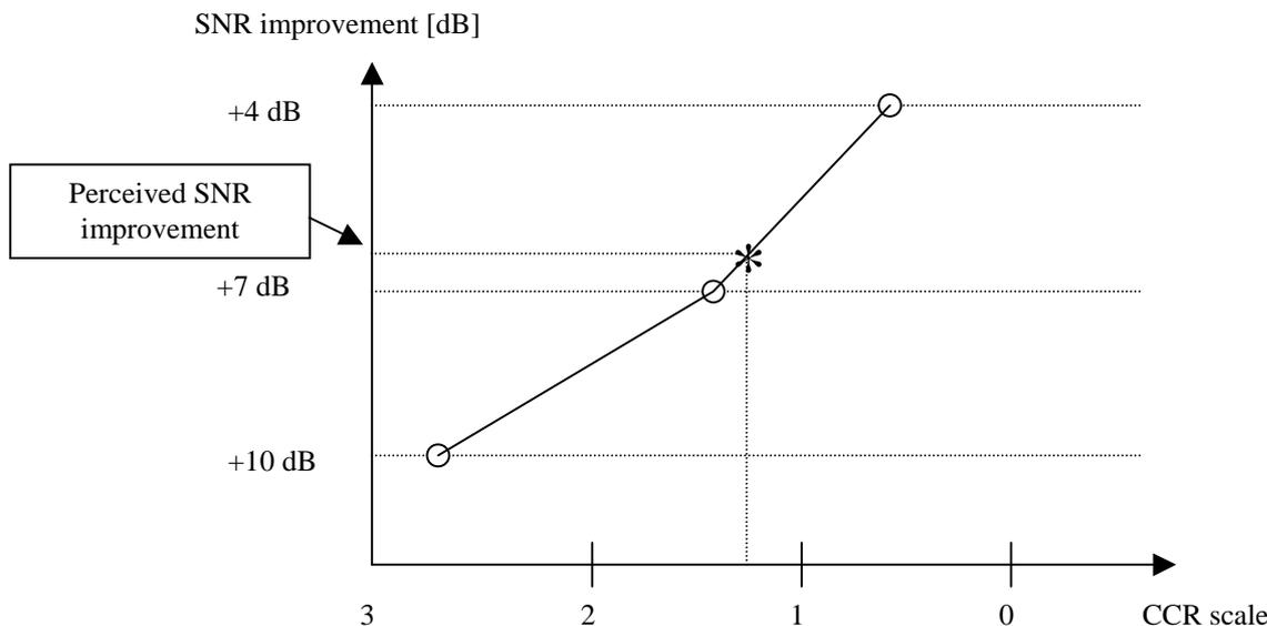
Figure D.1: Example of CCR versus SNR improvement graph
