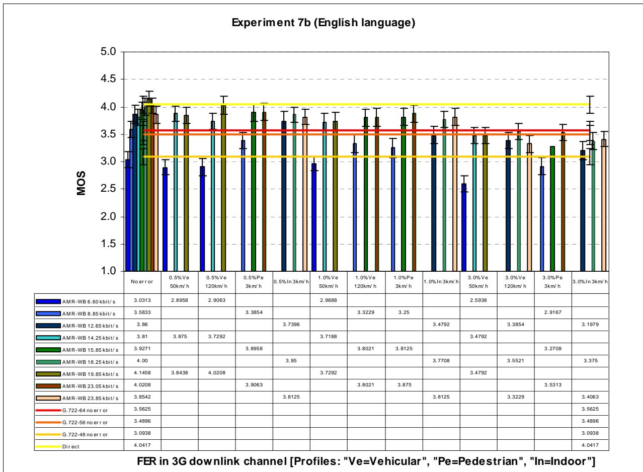
Figure 14.2: Experiment 7b, testing 3G downlink channel with English language
