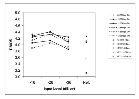
Figure 17.3a: Effects of Bit Rate, Input Level, and VAD/DTX 0n DMOS in the Dynastat Exp.1
