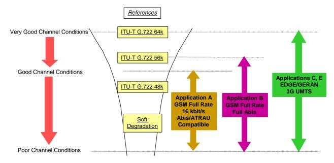
Figure 5.1: Quality requirements for the AMR-WB codec for the various applications [4].
