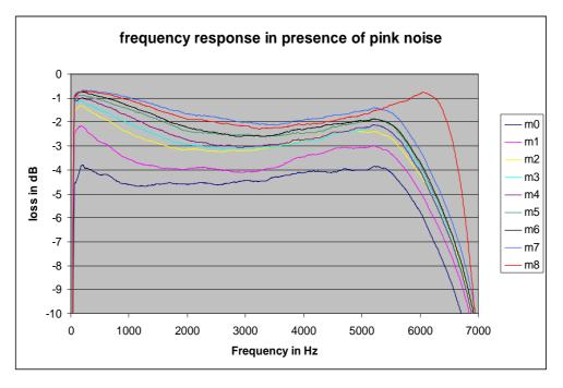
Figure 26.3: Frequency response of the AMR-WB codec (2nd method)
