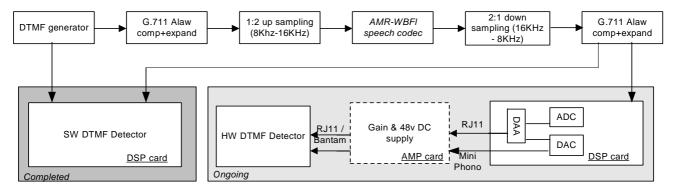
Figure B.6.1: DTMF Test Setup
