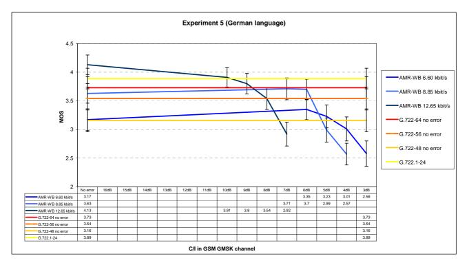
Figure 12.1: Experiment 5, testing GSM FR channel with German language
