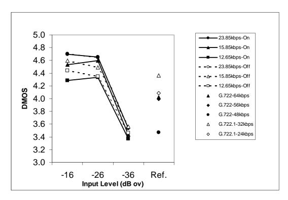
Figure 17.3b: Effects of Bit Rate, Input Level, and VAD/DTX on DMOS in the Nokia Exp.1
