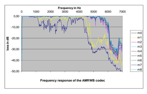
Figure 26.1: Frequency response of the AMR-WB codec (1st method)
