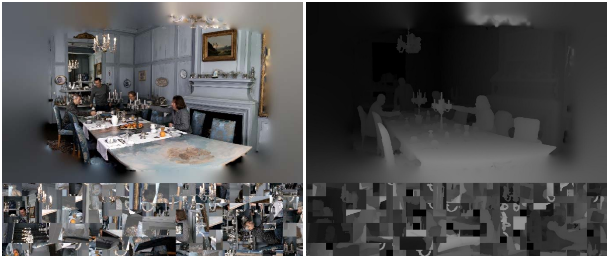
Figure 9.4.4.1.5.1-2: Video components of condition SCV with left texture and right geometry
