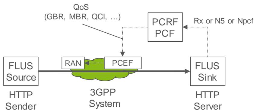
**Figure 10: HTTP based Architecture (or other OTT protocols)**
