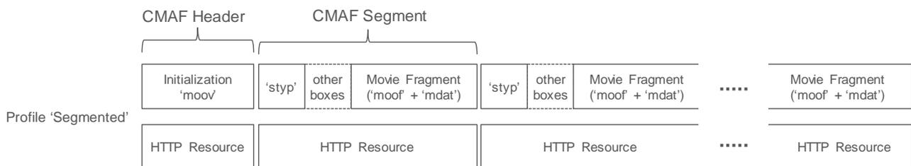
**Figure 3: Illustration of Segmented Profiles with one CMAF Chunk per CMAF Segment (with mapping to HTTP resources)**
