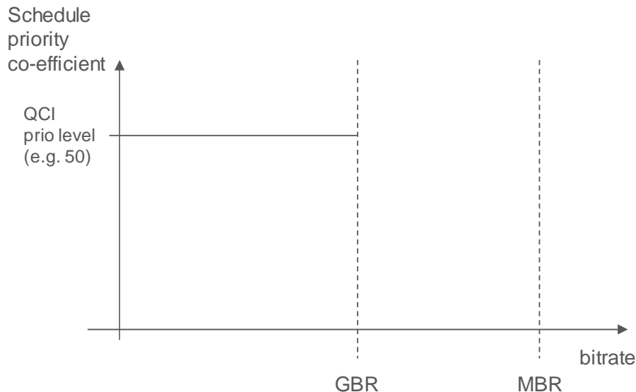
Figure 11: Today's prioritization: traffic gets priorities up to the GBR and is treated as best effort above GBR
