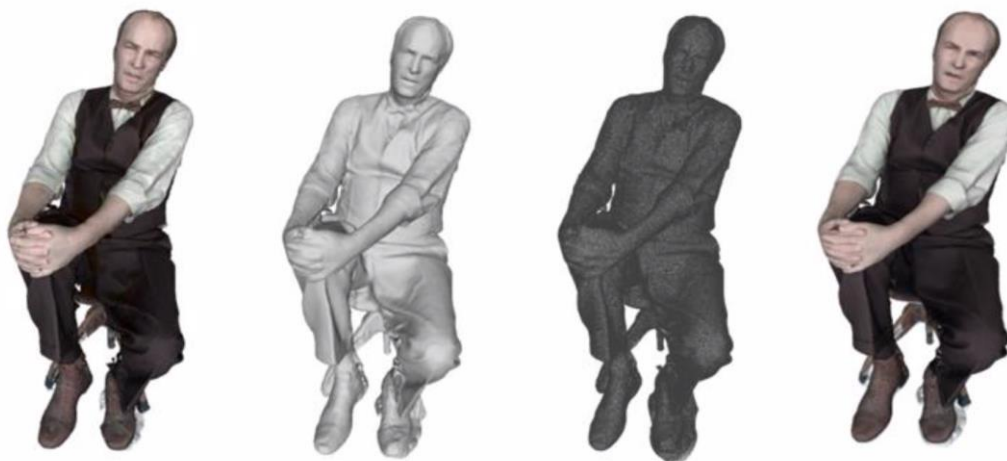
Figure 4.6.7-5: Example of resulting point cloud (left), and 3D models such as meshing, simplification and texturing (from second left to right)
