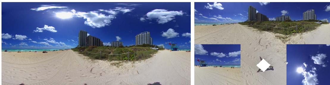
Figure 4.12: Equirectangular projection (left) vs Cubic mapping (right) of the same spherical content. Cube maps provide an approximately equal-area projection whereas equirectangular projection contains redundant samples towards poles of the image
