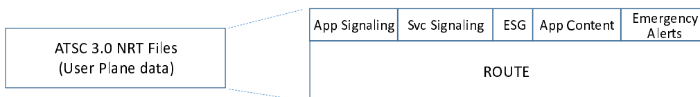
Figure 16: ATSC 3.0 NRT Service Protocol Stack over xMB-U
