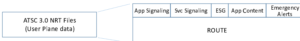
Figure 16: ATSC 3.0 NRT Service Protocol Stack over xMB-U
