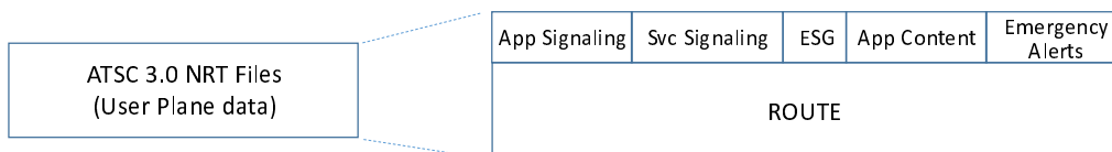
Figure 16: ATSC 3.0 NRT Service Protocol Stack over xMB-U
