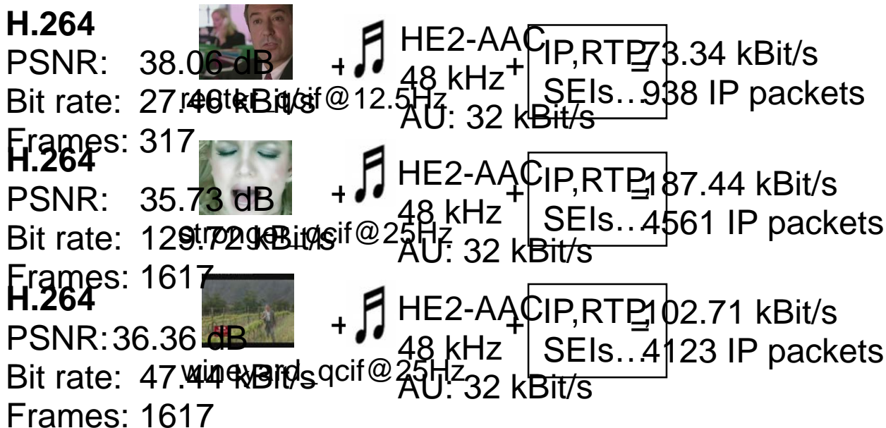
Figure 38: Video sequence parameters for H.264/AVC compliant base layer with GOP 16
