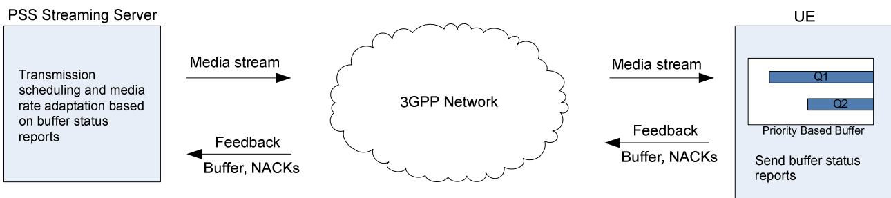
Figure 3: Transmission scheduling and media rate adaptation based on priority based buffer status reports
