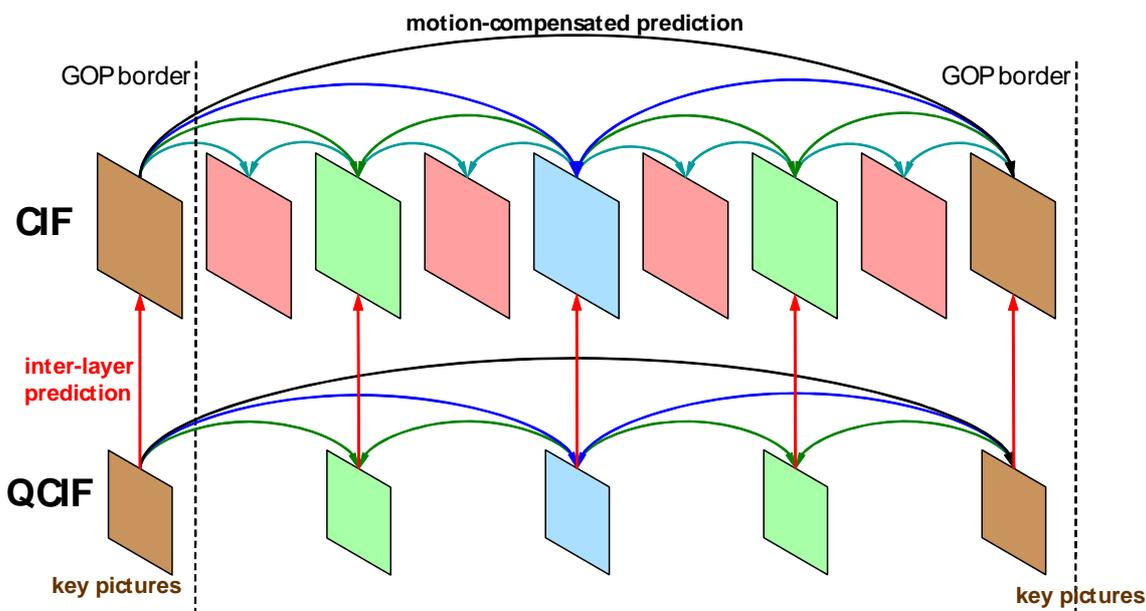
Figure 2: Example Prediction Structure for Spatial Scalability
