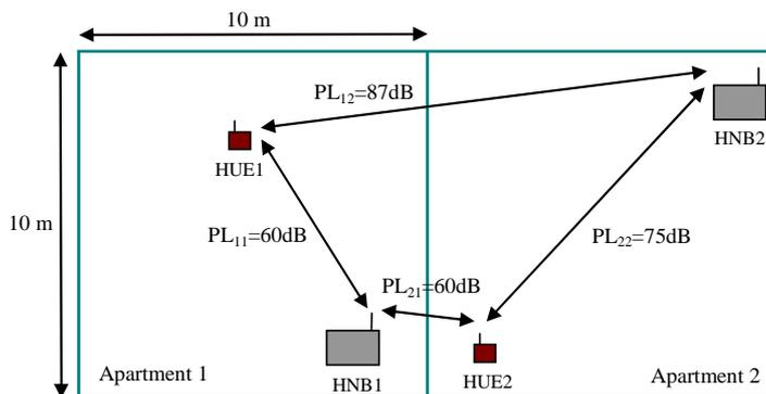
Figure 8.2.2.2-1: Inter-HNB uplink test set-up
