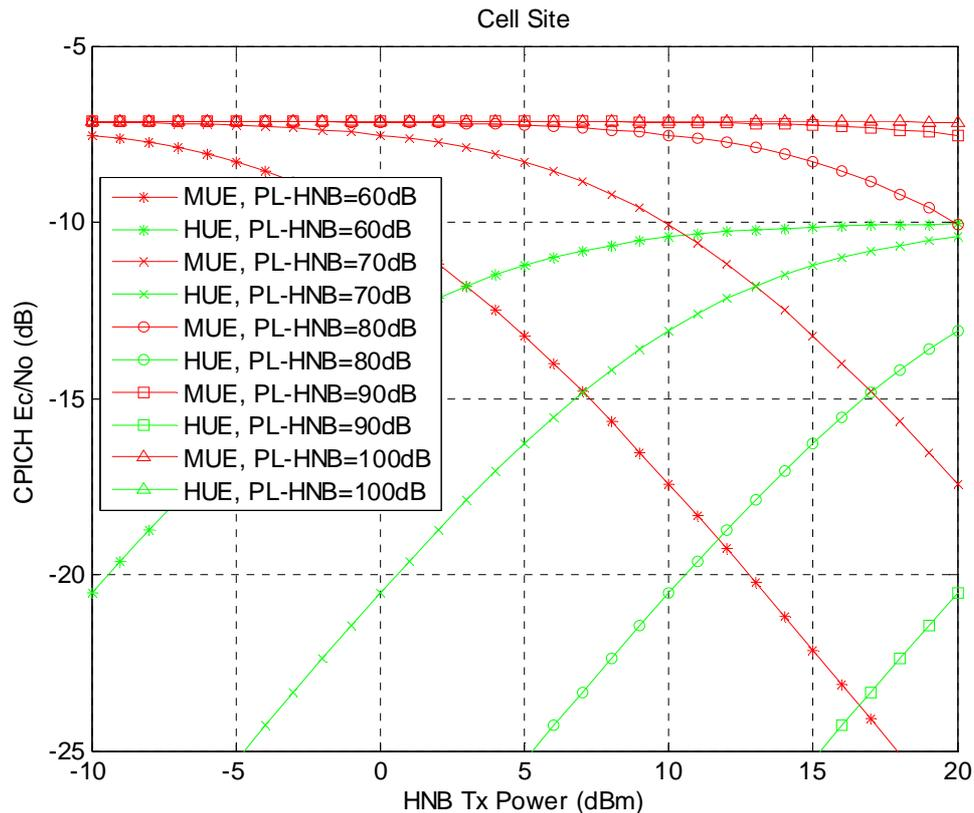
**Figure 7.2.1.1.1-3: Trade-off between HUE and MUE performance as a function of HNB tx power at cell site**
