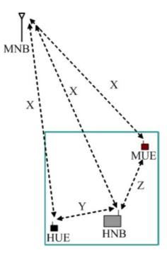
Figure 7.2.1.1-1: DL Interference Setup
