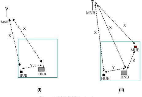
Figure 8.2.2.1-1: UL test setup
