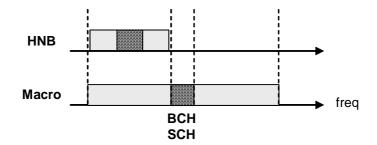
Figure 5.1.4-3 Spectrum arrangement for EUTRAN
