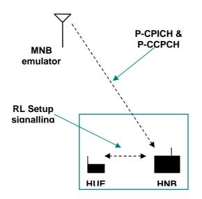
Figure 8.2-2: UL interference test setup
