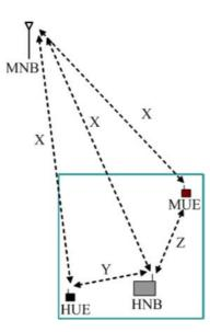
Figure 8.1-1: DL interference scenario
