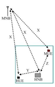
Figure 7.3.3.1-1: UL Interference Analysis Setup
