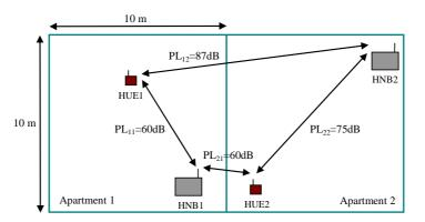
Figure 8.2.2.2-1: Inter-HNB uplink test set-up
