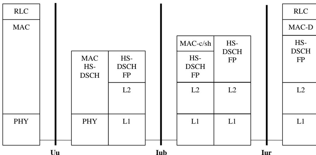
Figure 1: Radio Interface Protocol Architecture of HSDPA
