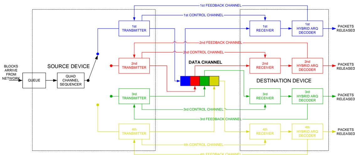
Figure 6: Single device example block diagram with quad channel stop-and-wait.
