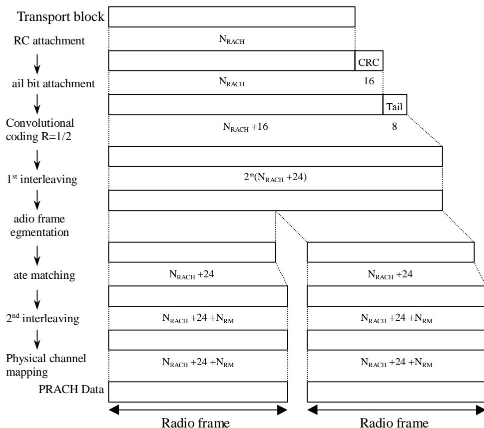
**Figure 16: Channel coding and multiplexing example for PRACH**
