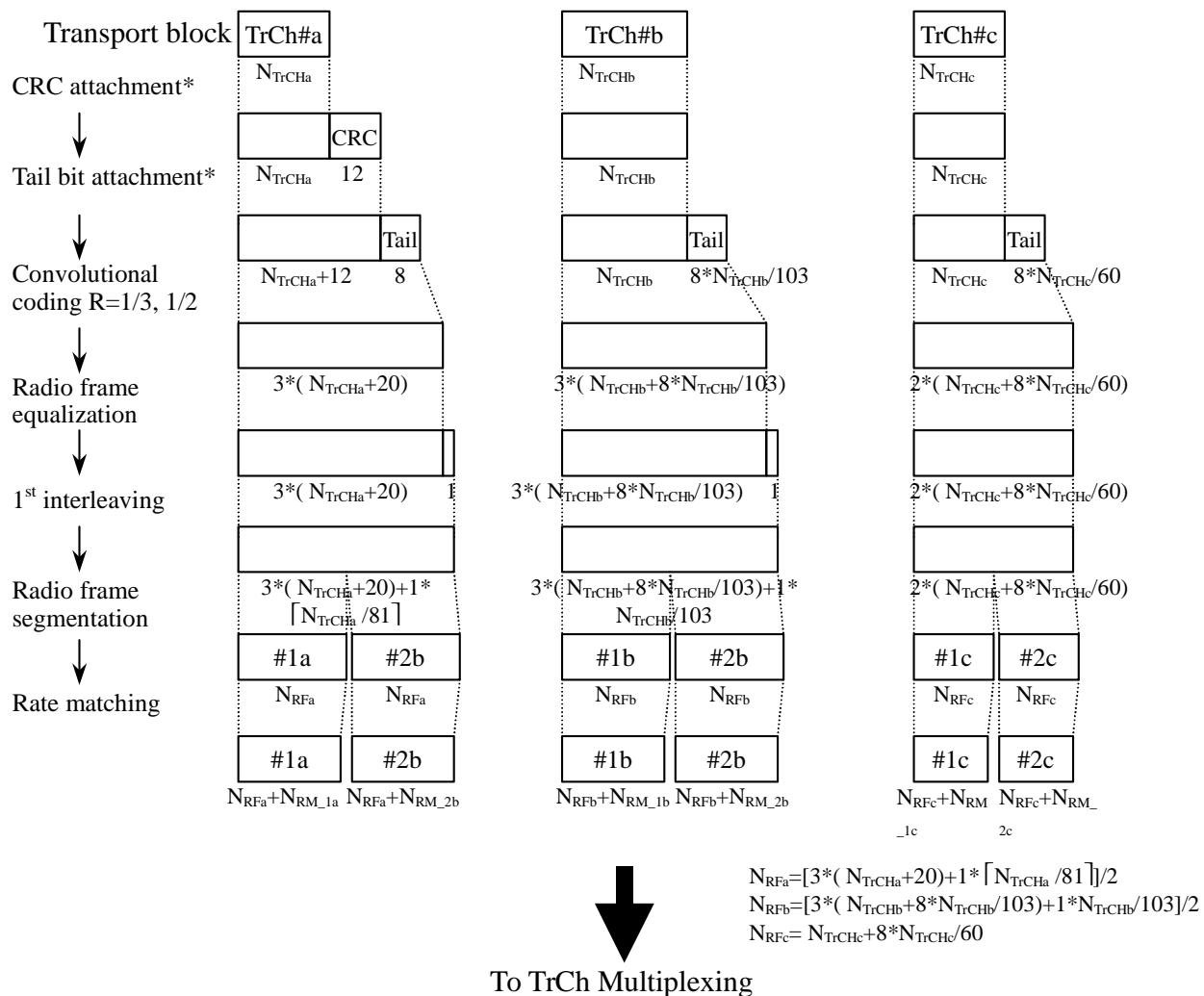
**Figure 18: Channel coding and multiplexing example for 12.2 kbps data**
