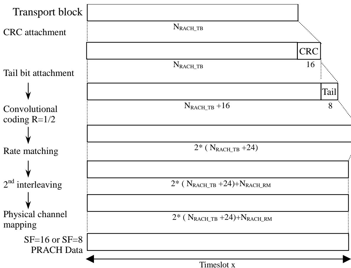
**Figure 44: Channel coding and multiplexing example for PRACH**
