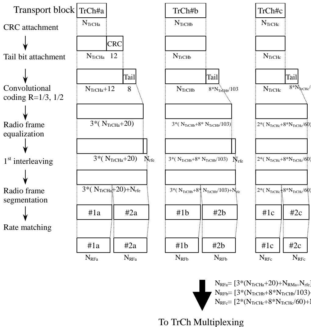
**Figure 32: Channel coding and multiplexing example for 12.2 kbps data**
