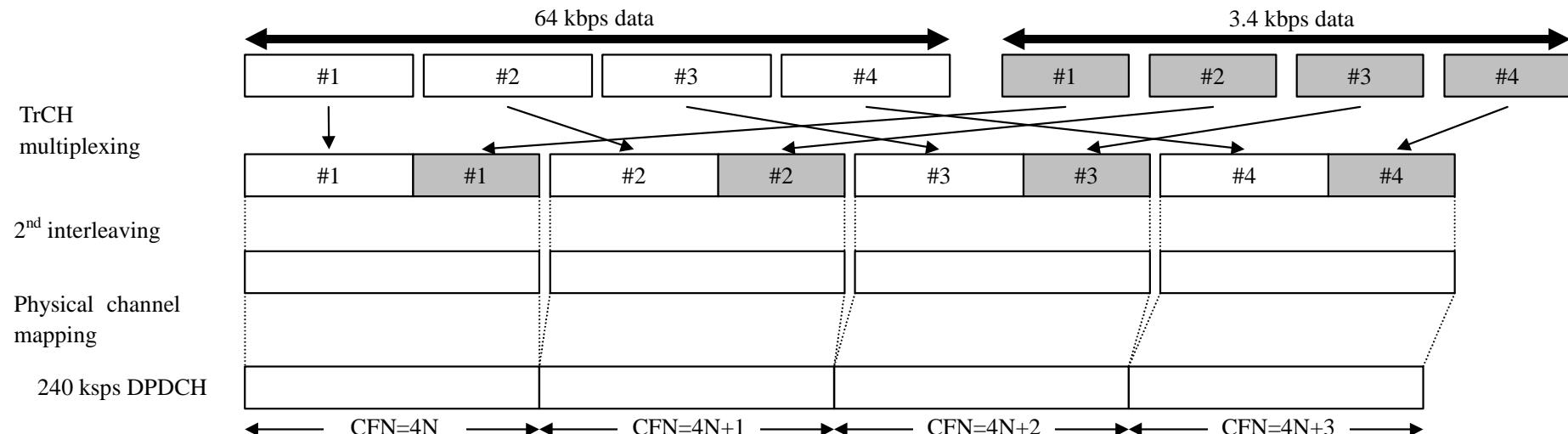
Figure 27: Channel coding and multiplexing example for multiplexing of 64 kbps data and 3.4 kbps data
