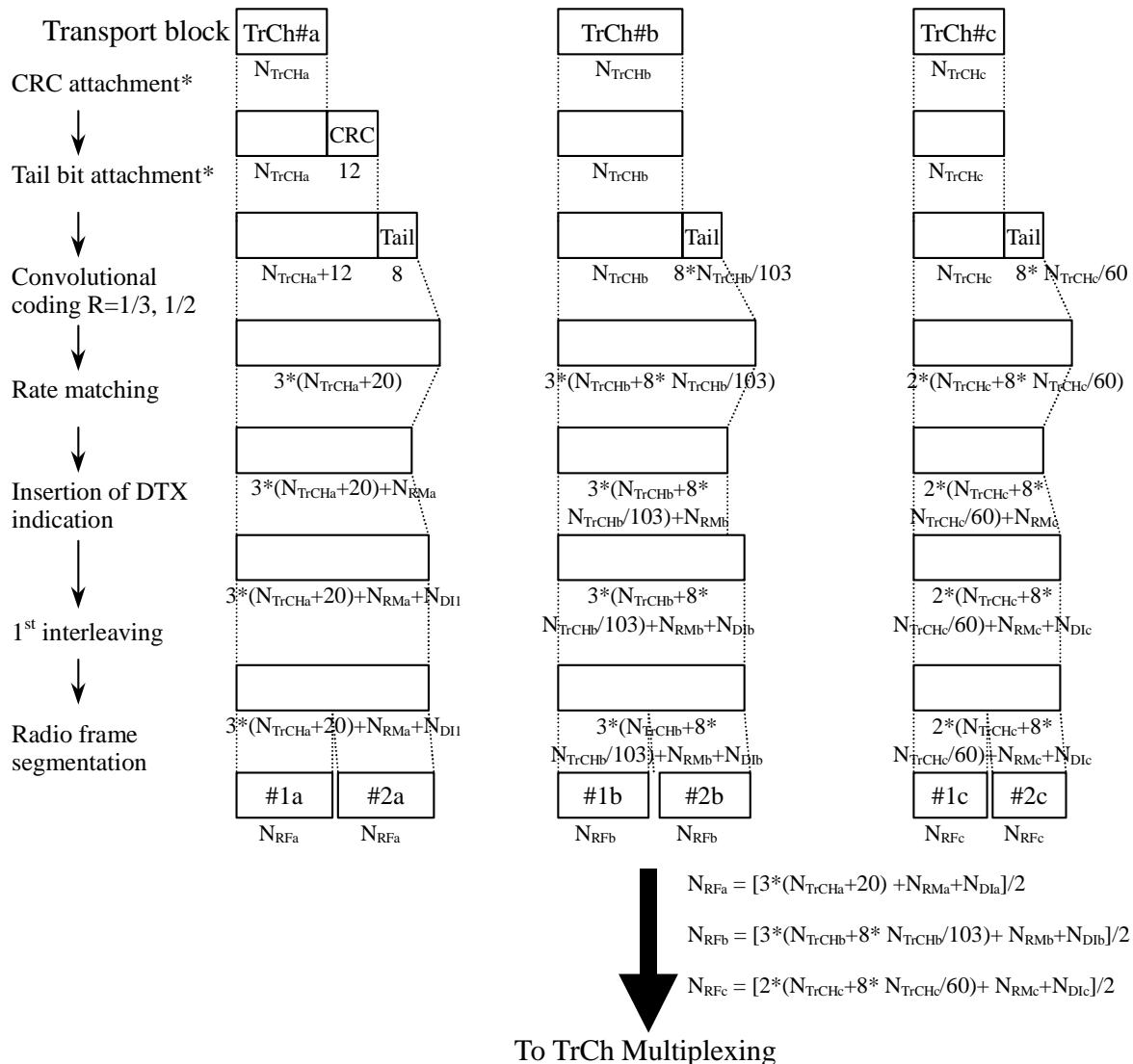
\* CRC and tail bits for TrCH#a is attached even if  $N_{TrCHa}=0$  bits since CRC parity bit attachment for 0 bit transport block is applied.
