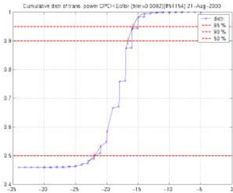
Figure 60: Cumulative distribution of transmission power DPCH_Ec/Ior when compressed mode is on. TGL = 14 slots
