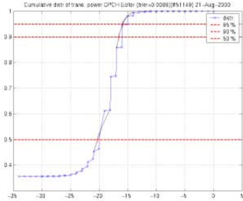
Figure 56: Cumulative distribution of transmission power DPCH_Ec/Ior when compressed mode is on. TGL = 4 slots
