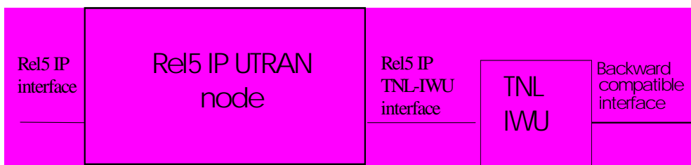
Figure 7-6: A TNL Interworking Unit present between the IP UTRAN Node and the ATM UTRAN Node
