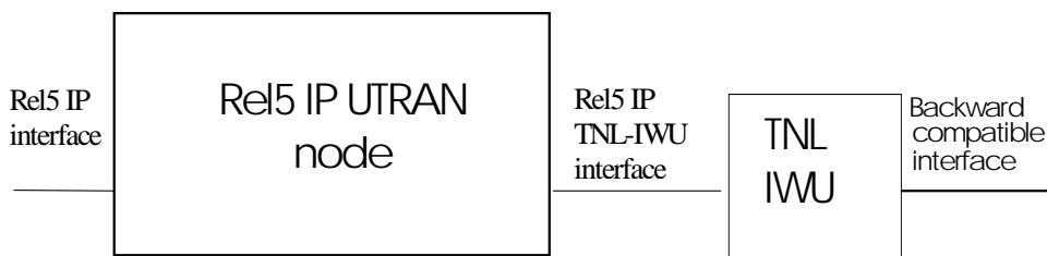
Figure 7-6: A TNL Interworking Unit present between the IP UTRAN Node and the ATM UTRAN Node
