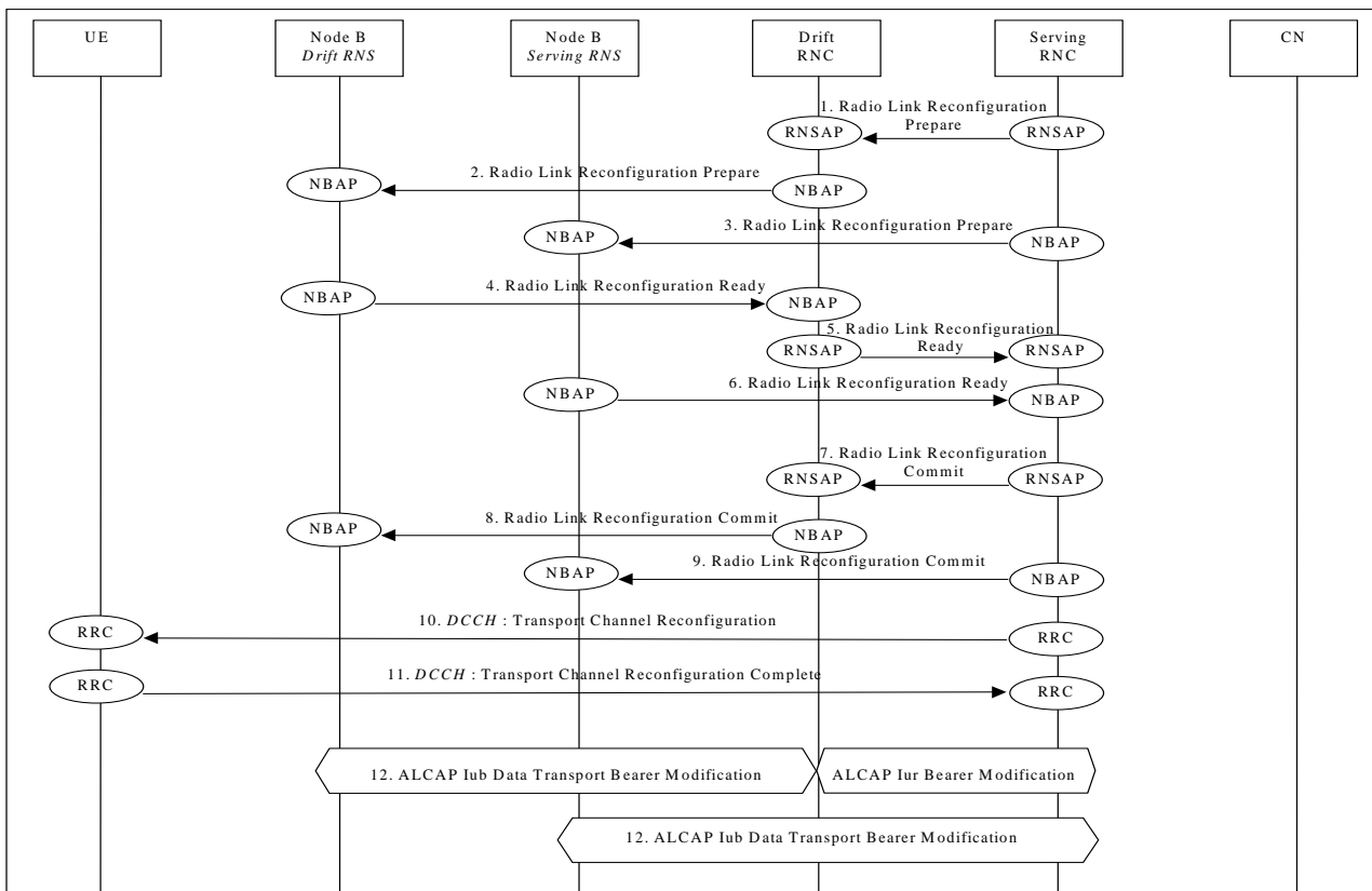
Figure 41b: Synchronised Transport Channel Reconfiguration, Bandwidth Decrease
