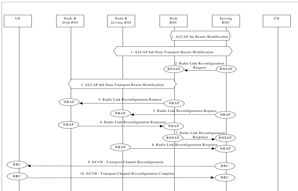
Figure 42a: Unsynchronised Transport Channel Reconfiguration, Bandwidth Increase
