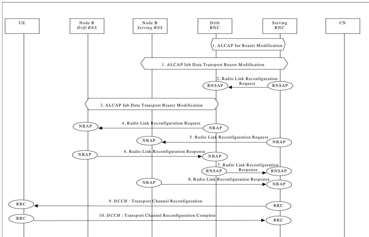
Figure 42a: Unsynchronised Transport Channel Reconfiguration, Bandwidth Increase
