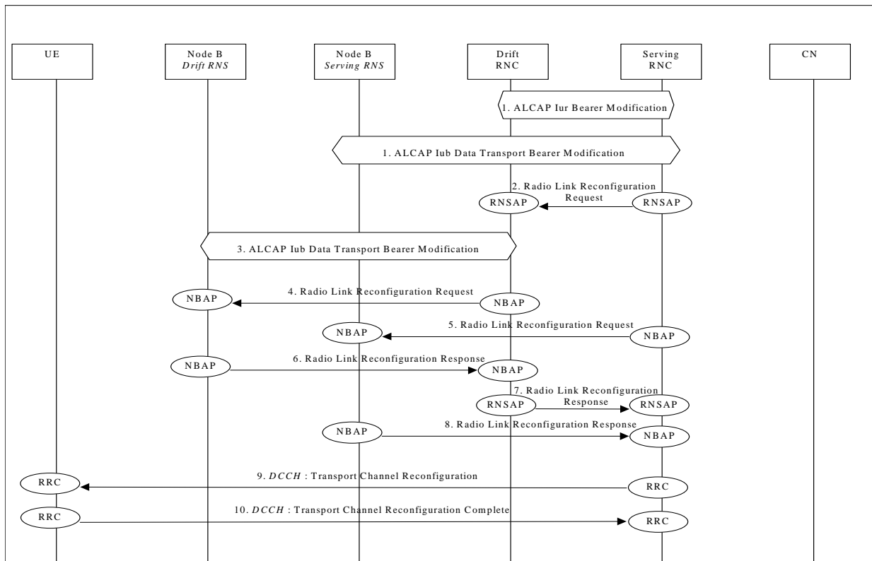
Figure 42a: Unsynchronised Transport Channel Reconfiguration, Bandwidth Increase
