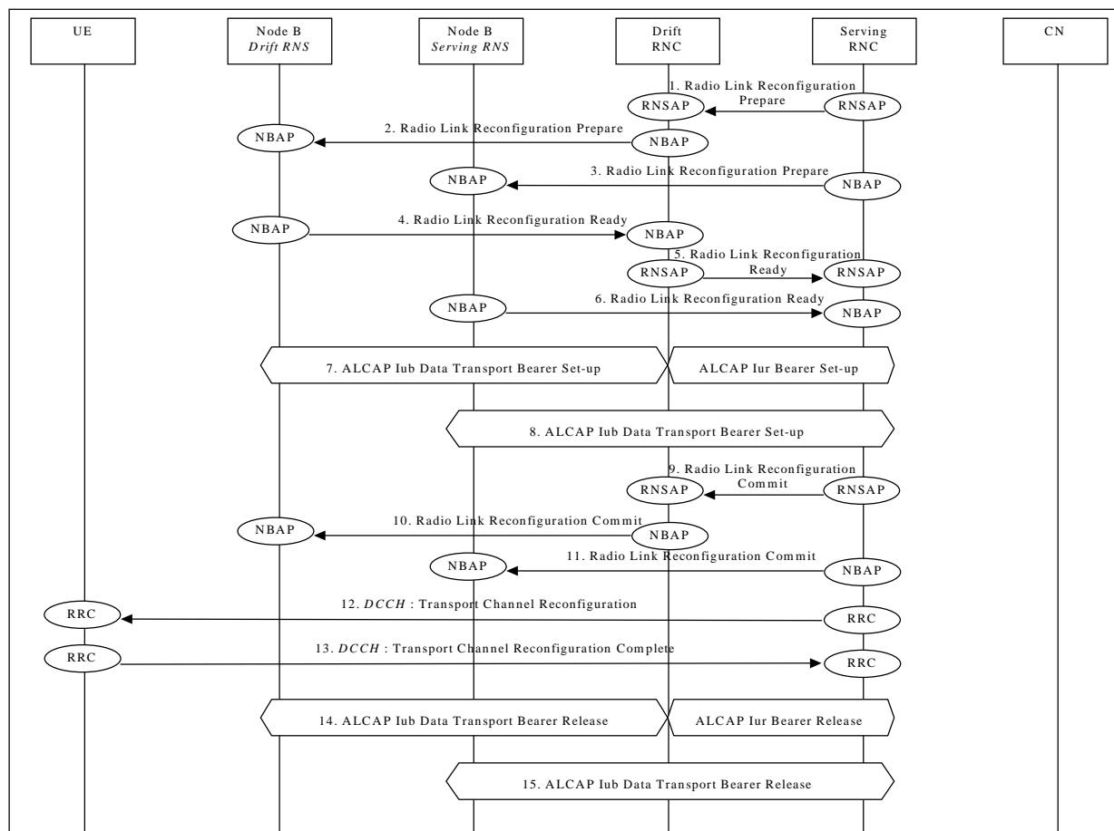
Figure 41: Synchronised Transport Channel Reconfiguration
