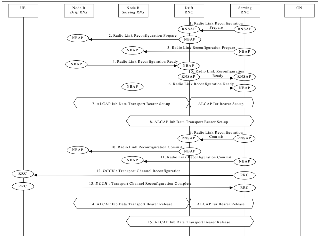
Figure 41: Synchronised Transport Channel Reconfiguration
