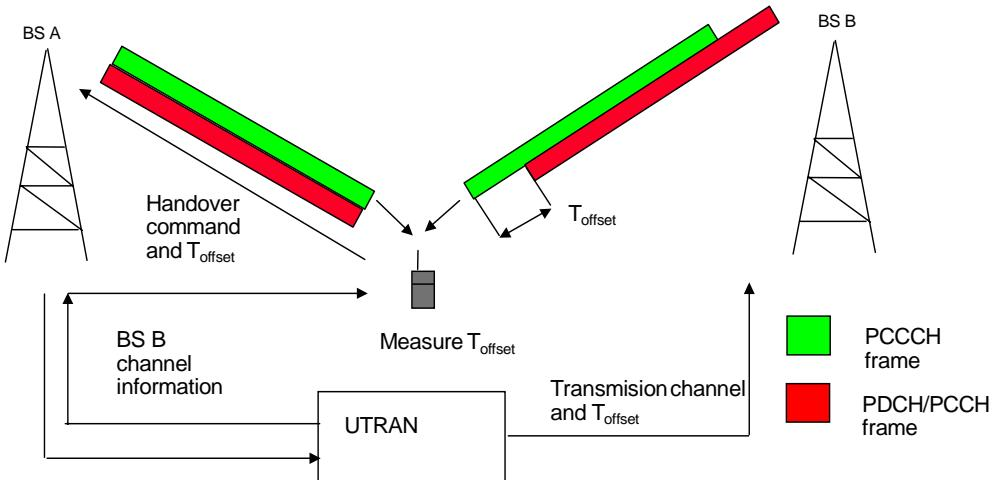
**Figure 5-2: Making transmissions capable to be combined in the Rake receiver from timing point of view**
