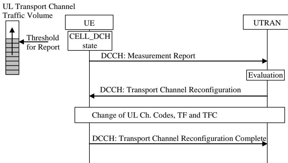
**Figure B-6: Transport channel reconfiguration triggered by increased UL data and configuration in UTRAN DL**
