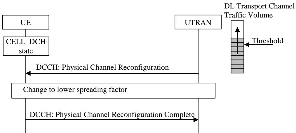
**Figure B-3: Physical channel reconfiguration triggered by increased DL data and configuration in UTRAN DL**
