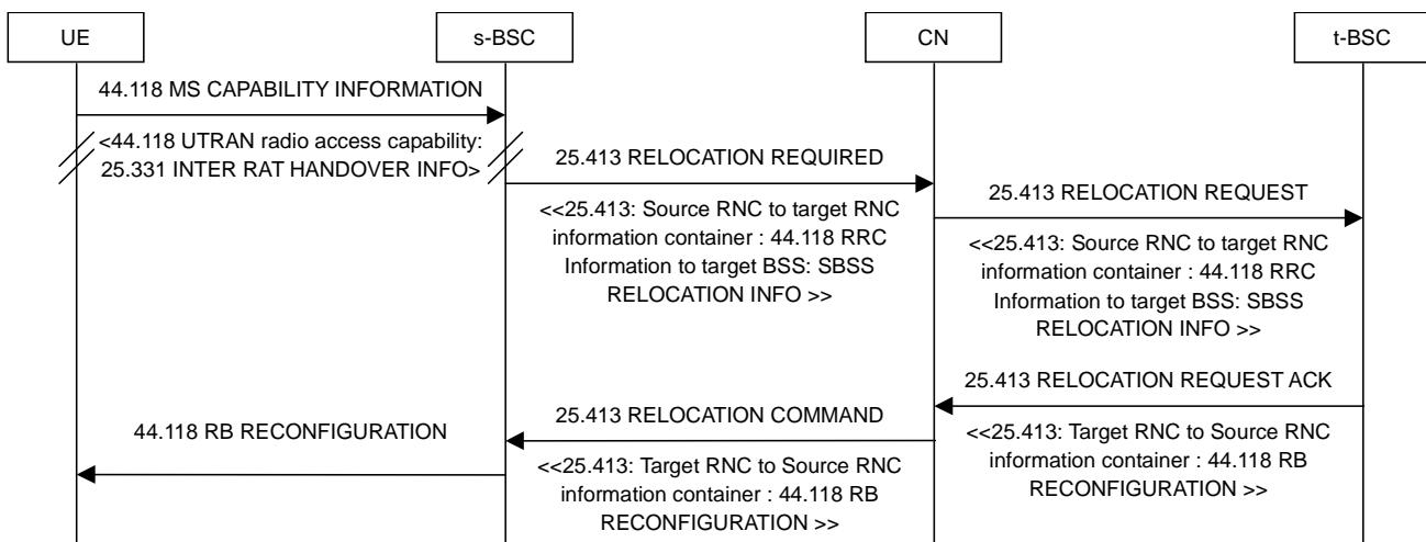
**Figure 5.1.7.2-4a: SBSS relocation, GERAN Iu mode, normal flow**
