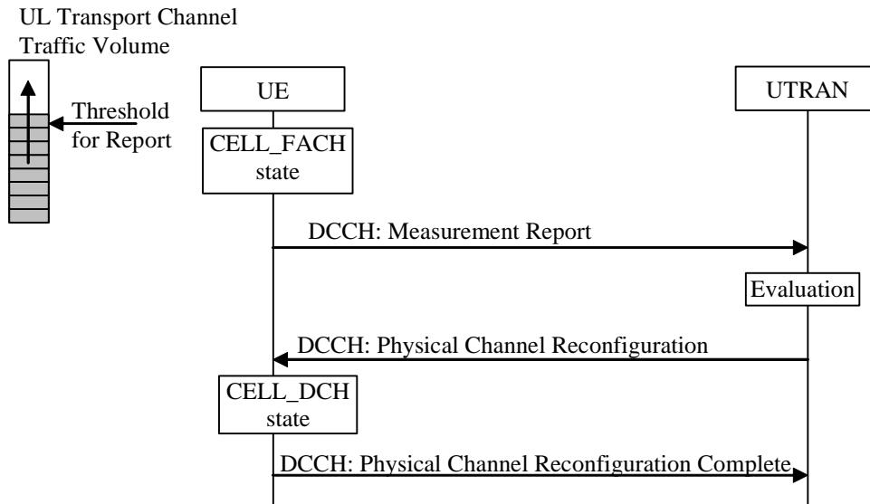
**Figure B-2: Physical channel reconfiguration triggered by increased UL data and with a switch from CELL\_FACH to CELL\_DCH**
