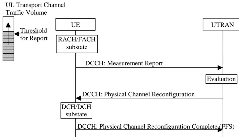
**Figure B-2: Physical channel reconfiguration triggered by increased UL data and with a switch from RACH/FACH to DCH/DCH**
