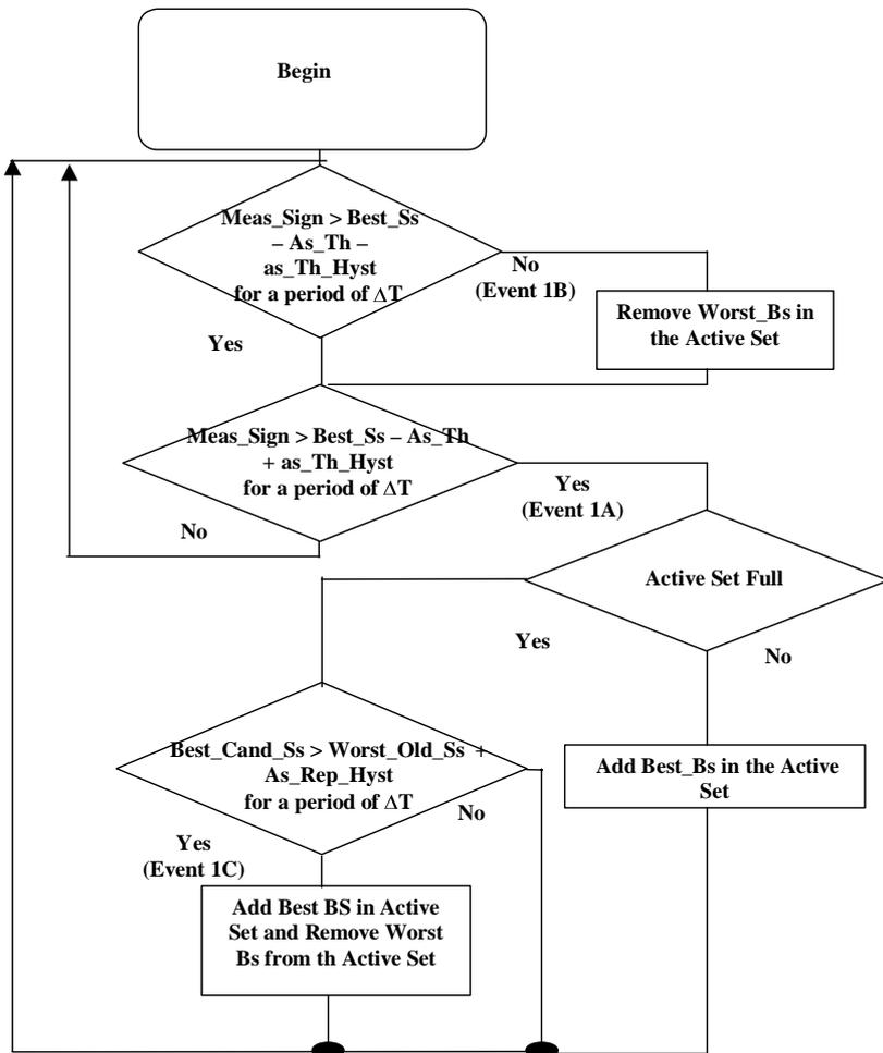
Figure C-1: flow-chart of a Soft Handover algorithm
