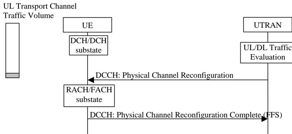
**Figure B-5: Physical channel reconfiguration triggered by decreased UL data and with a switch from DCH/DCH to RACH/FACH**
