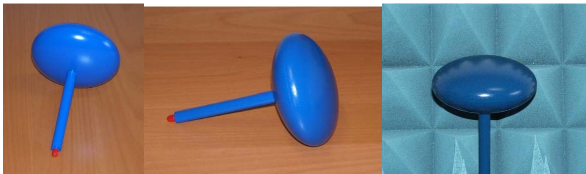
Figure 7.7 Examples of reference magnetic dipoles (loop antennas) [41].
