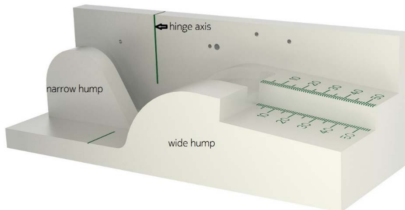
Figure 5.1.6.2-1 Alignment Tool B and right-handed fold hand phantom with a spacer. Use left-handed (mirror-imaged) spacers with left-handed phantoms.
