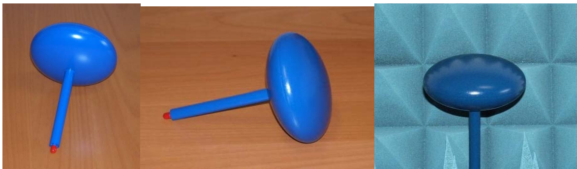
Figure 7.7 Examples of reference magnetic dipoles (loop antennas) [41].
