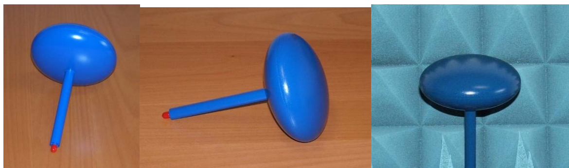
Figure 7.7 Examples of reference magnetic dipoles (loop antennas) [41].
