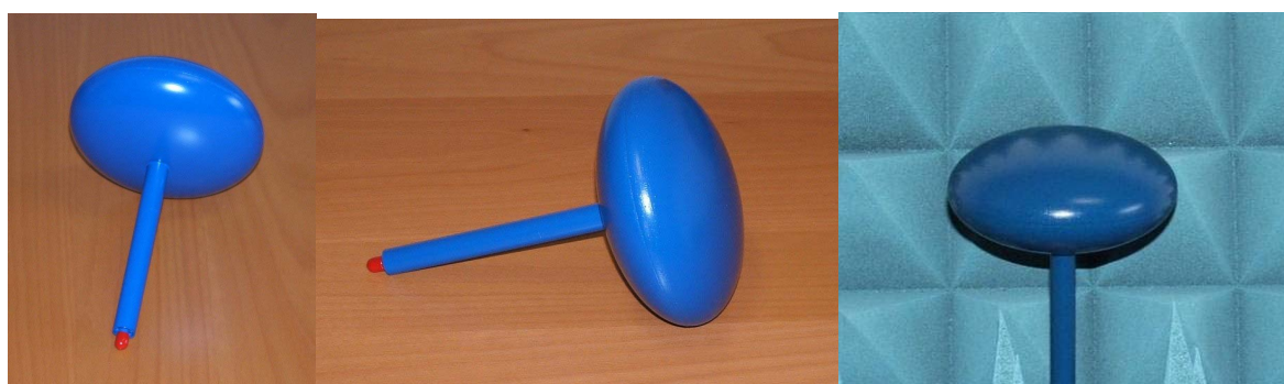
Figure 7.7 Examples of reference magnetic dipoles (loop antennas) [41].
