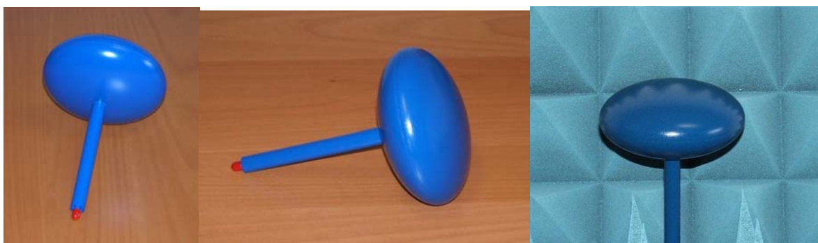
Figure 7.7 Examples of reference magnetic dipoles (loop antennas) [41].
