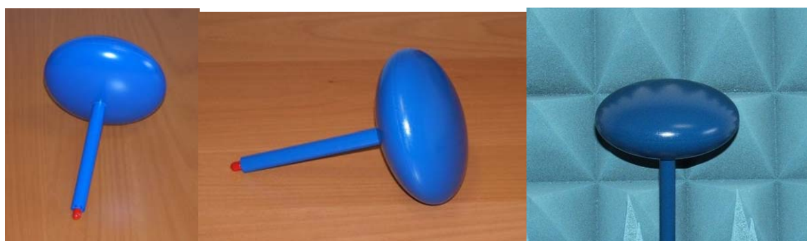
Figure 7.7 Examples of reference magnetic dipoles (loop antennas) [41].
