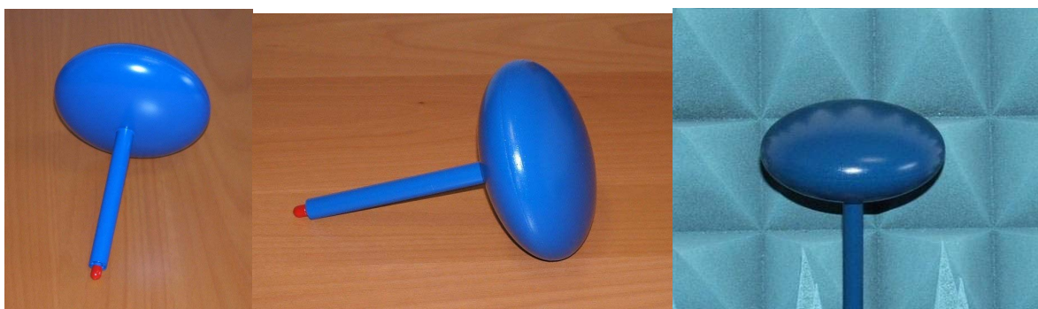
Figure 7.7 Examples of reference magnetic dipoles (loop antennas) [41].
