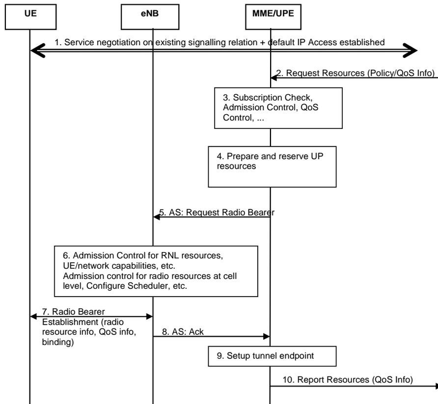
**Figure 9.3: Information flow for Resource Establishment in the Radio Network for application level signalling**
