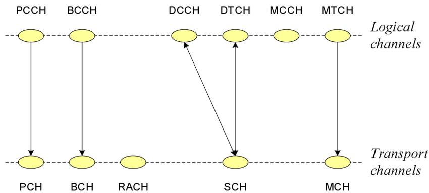
**Figure 8.3: Mapping between logical channels and transport channels**
