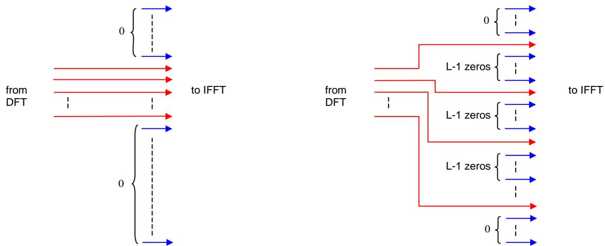
**Figure 7.3: Localized mapping (left) and distributed mapping (right).**
