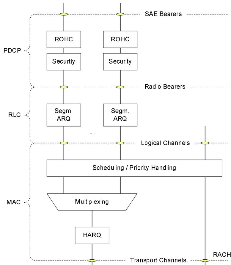
Figure 8.2: Layer 2 Structure for UL in UE
