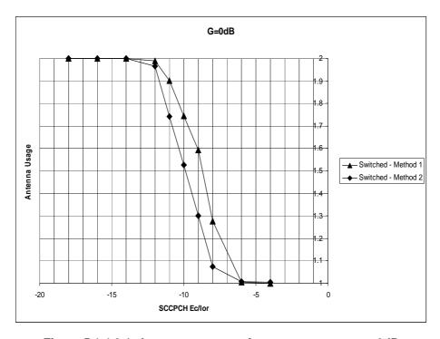
Figure 5.1.4.2.4: Antenna usage performance, geometry = 0dB
