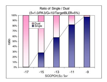
Fig. 5.1.4.1.4 Ratio between 1 and 2 antenna in PA3 ( $\delta$ =1.0).
