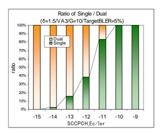
Fig. 5.1.4.1.9 Ratio between 1 and 2 antenna in VA3 ( $\delta$ =1.5).
