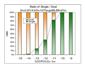
Fig. 5.1.4.1.10 Ratio between 1 and 2 antenna in VA3 ( $\delta$ =3.0)
