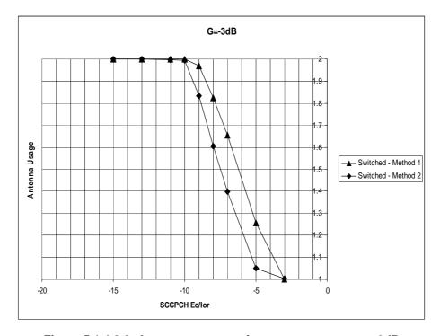
Figure 5.1.4.2.2: Antenna usage performance, geometry = -3dB
