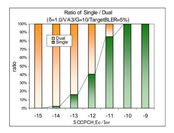
Fig. 5.1.4.1.8 Ratio between 1 and 2 antenna in VA3 ( $\delta$ =1.0).
