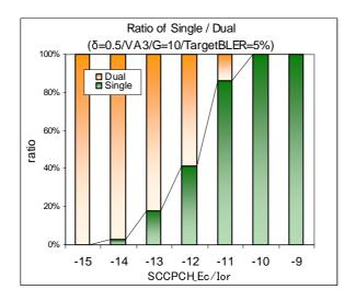
Fig. 5.1.4.1.7 Ratio between 1 and 2 antenna in VA3 ( $\delta$ =0.5).
