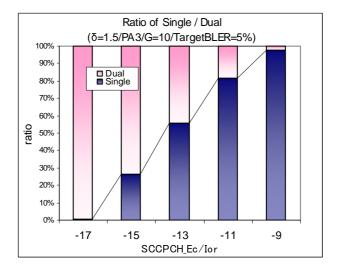
Fig. 5.1.4.1.5 Ratio between 1 and 2 antenna in PA3 ( $\delta$ =1.5).
