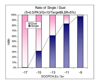
Fig. 5.1.4.1.3 Ratio between 1 and 2 antenna in PA3 ( $\delta$ =0.5).
