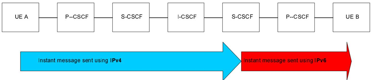
**Figure 5-12b: Example with dual stack IM CN subsystem and Immediate Messaging (terminating S-CSCF is dual stack)**
