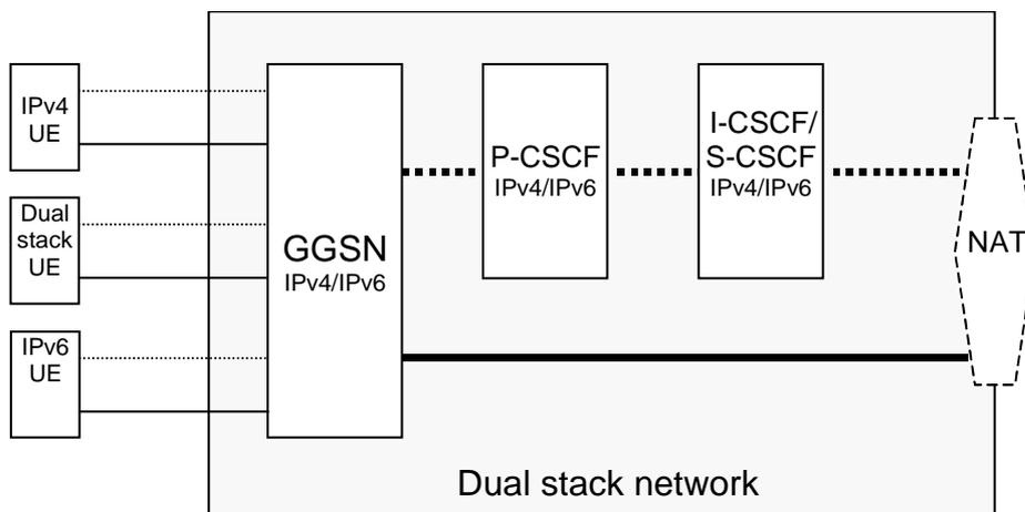
**Figure 5-3: Non-roaming dual Stack IM CN subsystem**
