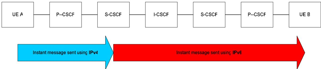
**Figure 5-12a: Example with dual stack IM CN subsystem and Immediate Messaging (originating S-CSCF is dual stack)**
