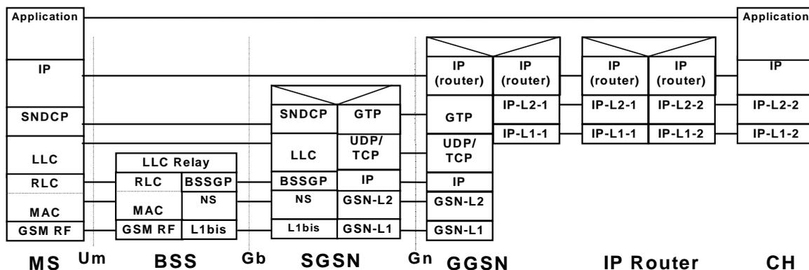
Figure 8.6a: Protocol stack for GPRS including the Internet
