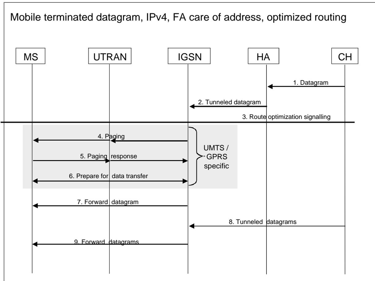
Figure 11.7.2b: Delivery of mobile terminated datagrams, optimised routing
