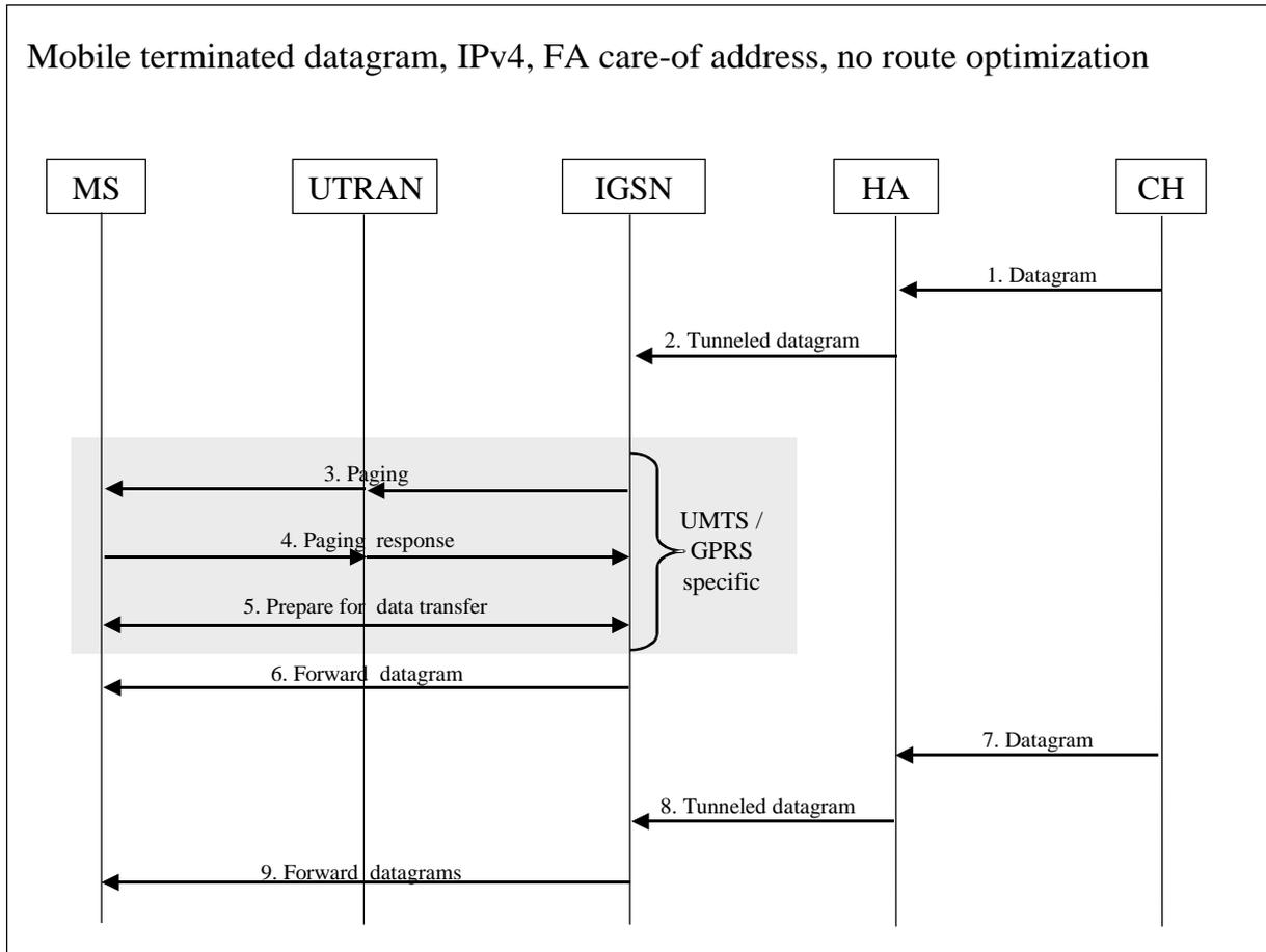
Figure 11.7.2a: Delivery of mobile terminated datagrams, no route optimisation
