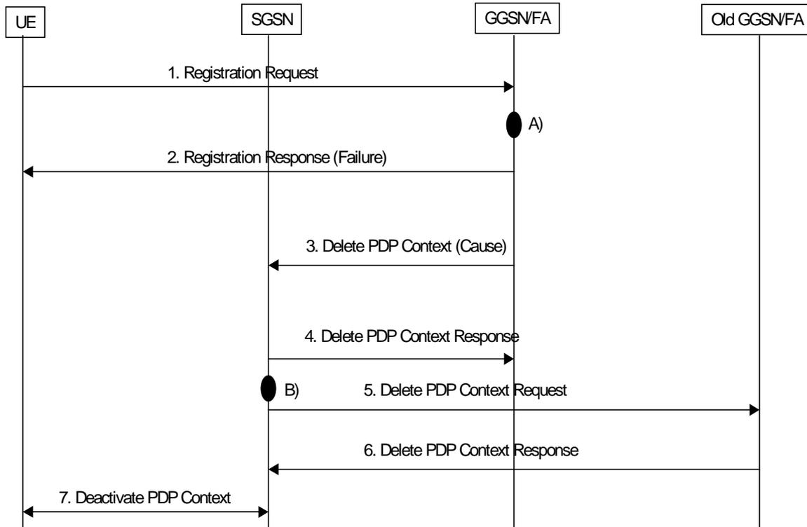
**Figure 10.2b: Case when no fall-back is possible**
