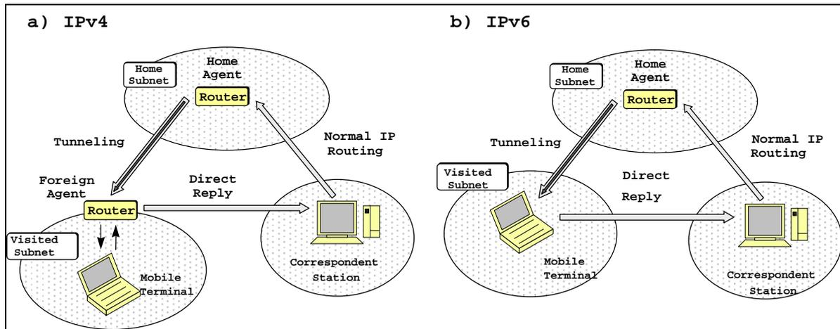
Figure A.1: Basic architecture for supporting IP mobility
