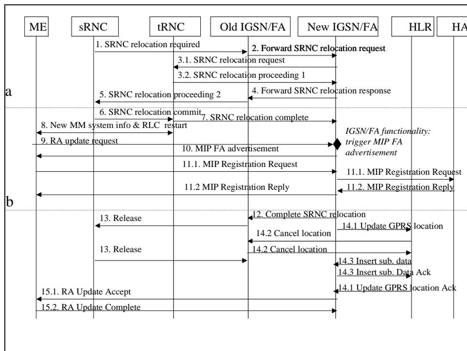
Figure 11.6a: SRNS relocation in a step 3 network
