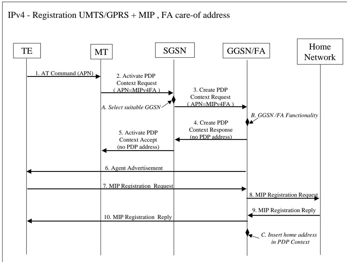
**Figure 9.4a, PDP Context activation with Mobile IP(+) registration (the PPP setup and UMTS/GPRS attach procedure not included)**
