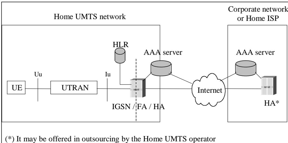
Figure 8.7.1a: UE attached to the Home UMTS operator
