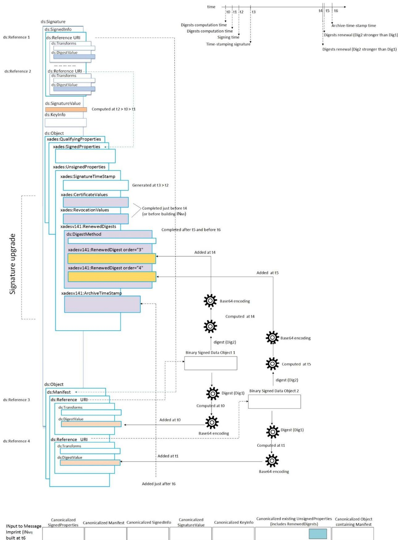
Figure A.3: Using xadesv141:RenewedDigests for countering signed detached objects substitution attack
