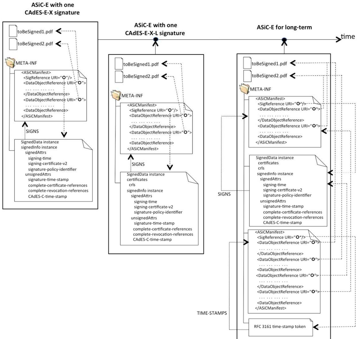
**Figure 21: Transitions for an ASiC-E with one CADES-E-X to an ASiC-E with one CADES-E-X-L signature and to an ASiC-E with availability and integrity of validation material**
