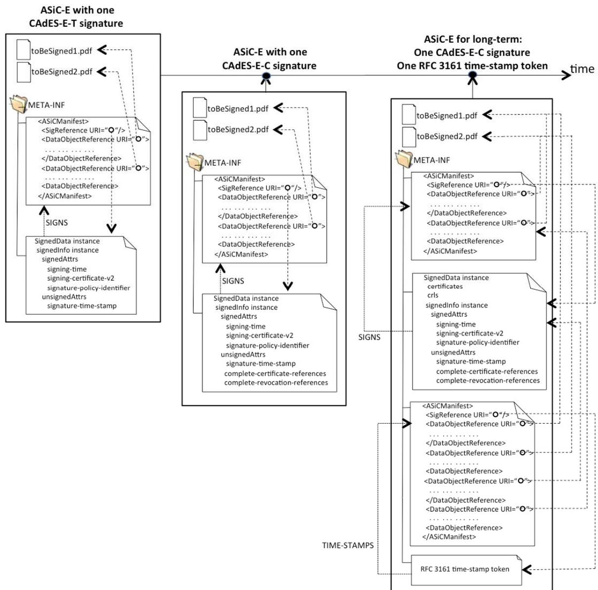
**Figure 18: Transitions for an ASiC-E with one CADES-E-T signature up to ASiC-E with availability and integrity of validation material**
