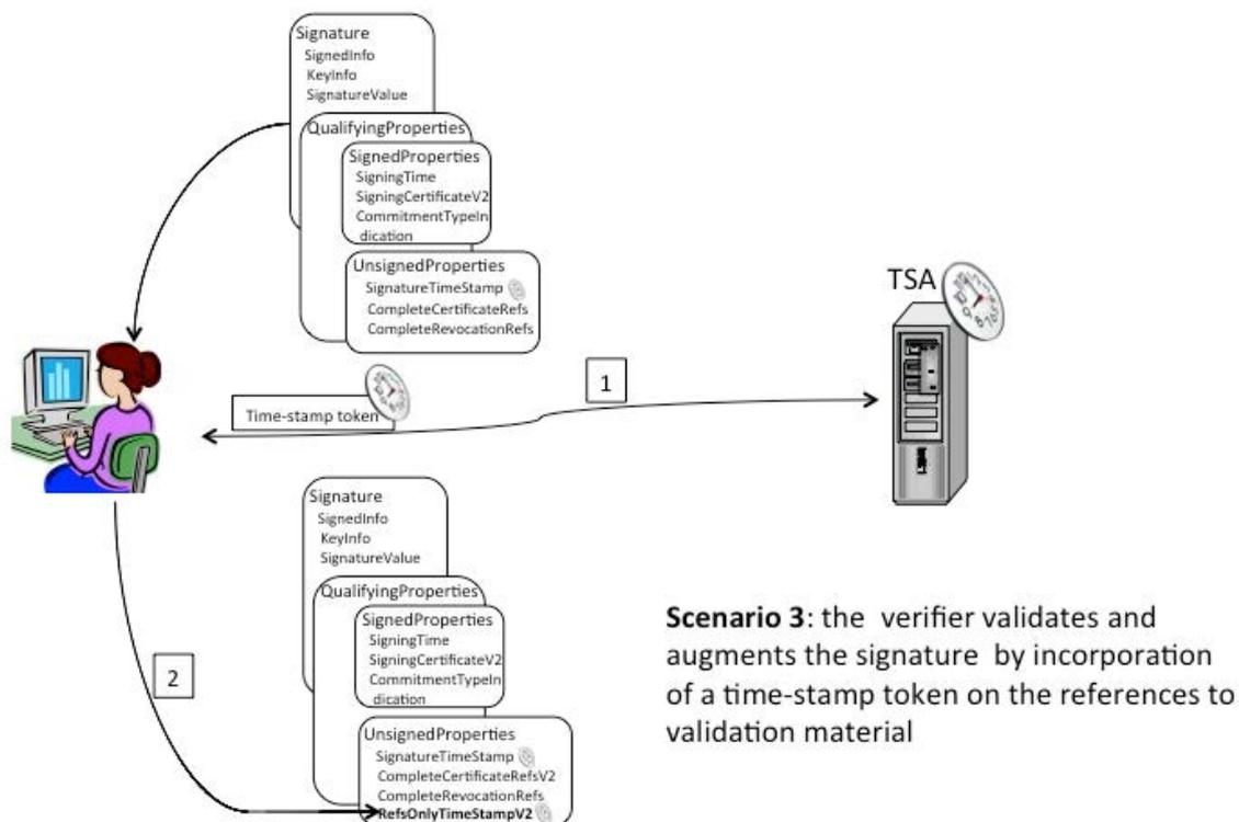
**Figure 4: Verifier validating a signature with unsigned properties/attributes, requesting time-stamp token on references to validation material, and augmenting the signature with this time-stamp token**
