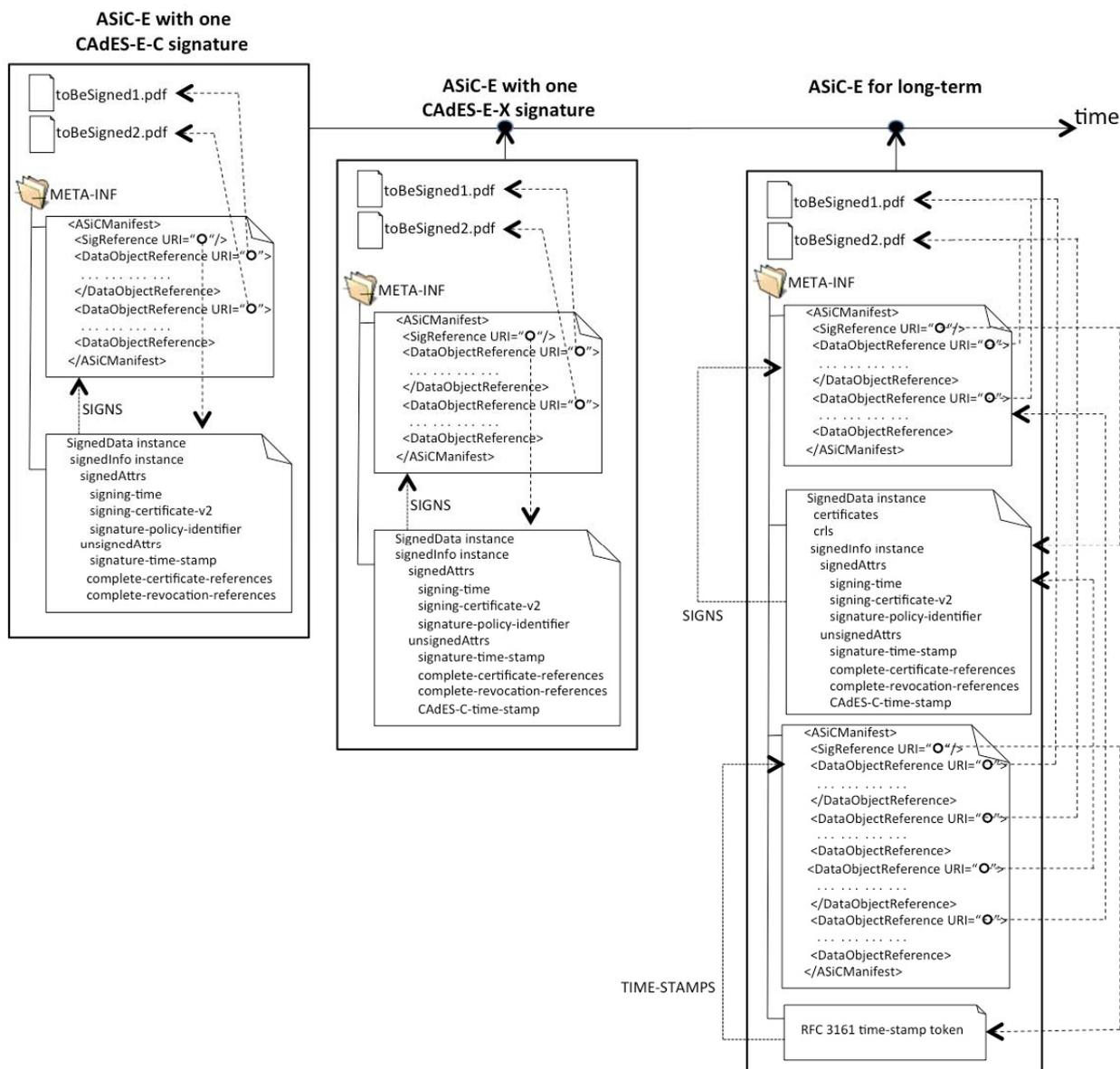
**Figure 20: Transitions for an ASiC-E with one CADES-E-C to an ASiC-E with one CADES-E-X signature and to an ASiC-E with availability and integrity of validation material**
