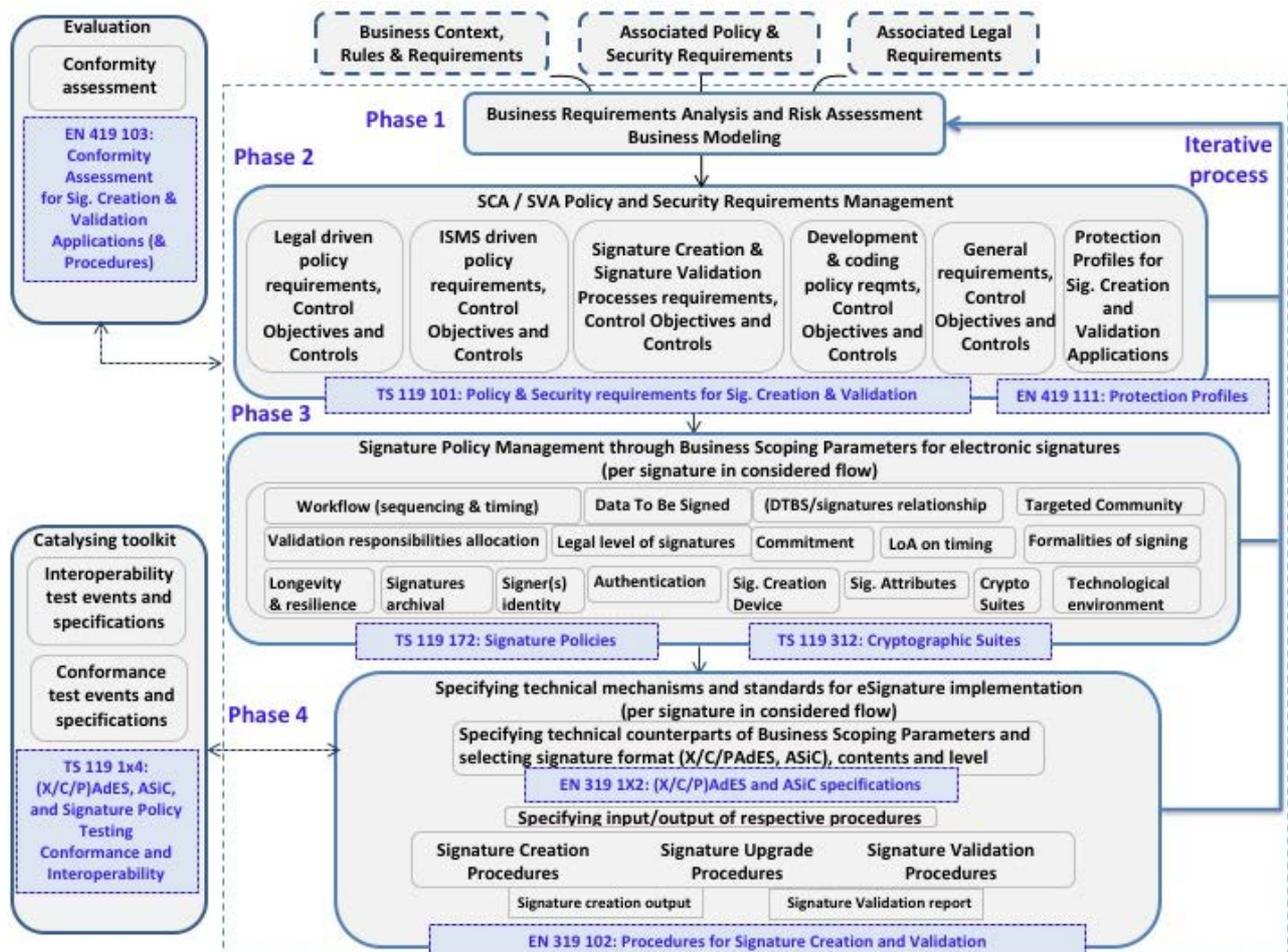
Figure 22: Relationship between process' tasks and documents within the area 1 of the Rationalized Framework
