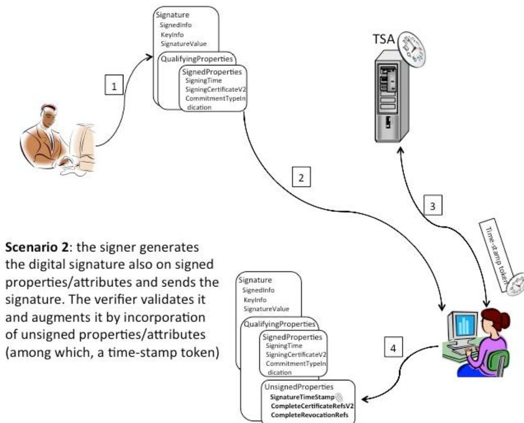
**Figure 3: Signer generating the signature, verifier validating it, requesting time-stamp token on the digital signature value, and augmenting it with unsigned properties/attributes**
