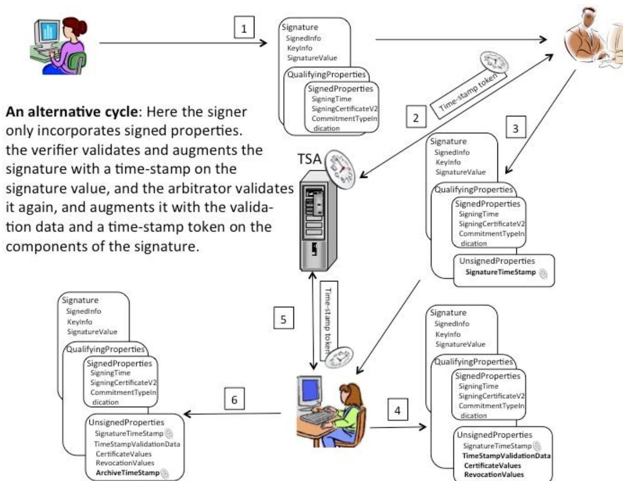
**Figure 7: Alternative signature lifecycle resulting in augmented signature without references to validation material**
