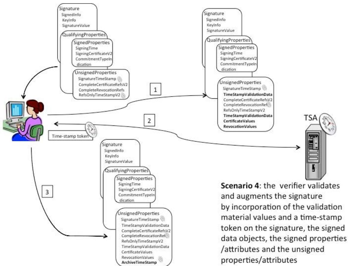
**Figure 5: Verifier validating a signature with unsigned properties/attributes, requesting an archive time-stamp token, and augmenting the signature with the validation material and the archive time-stamp token**
