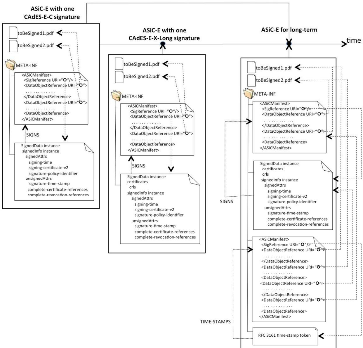
**Figure 19: Transitions from an ASiC-E with one CADES-E-C signature up to ASiC-E with availability and integrity of validation material, without time-stamp tokens on references to validation material**
