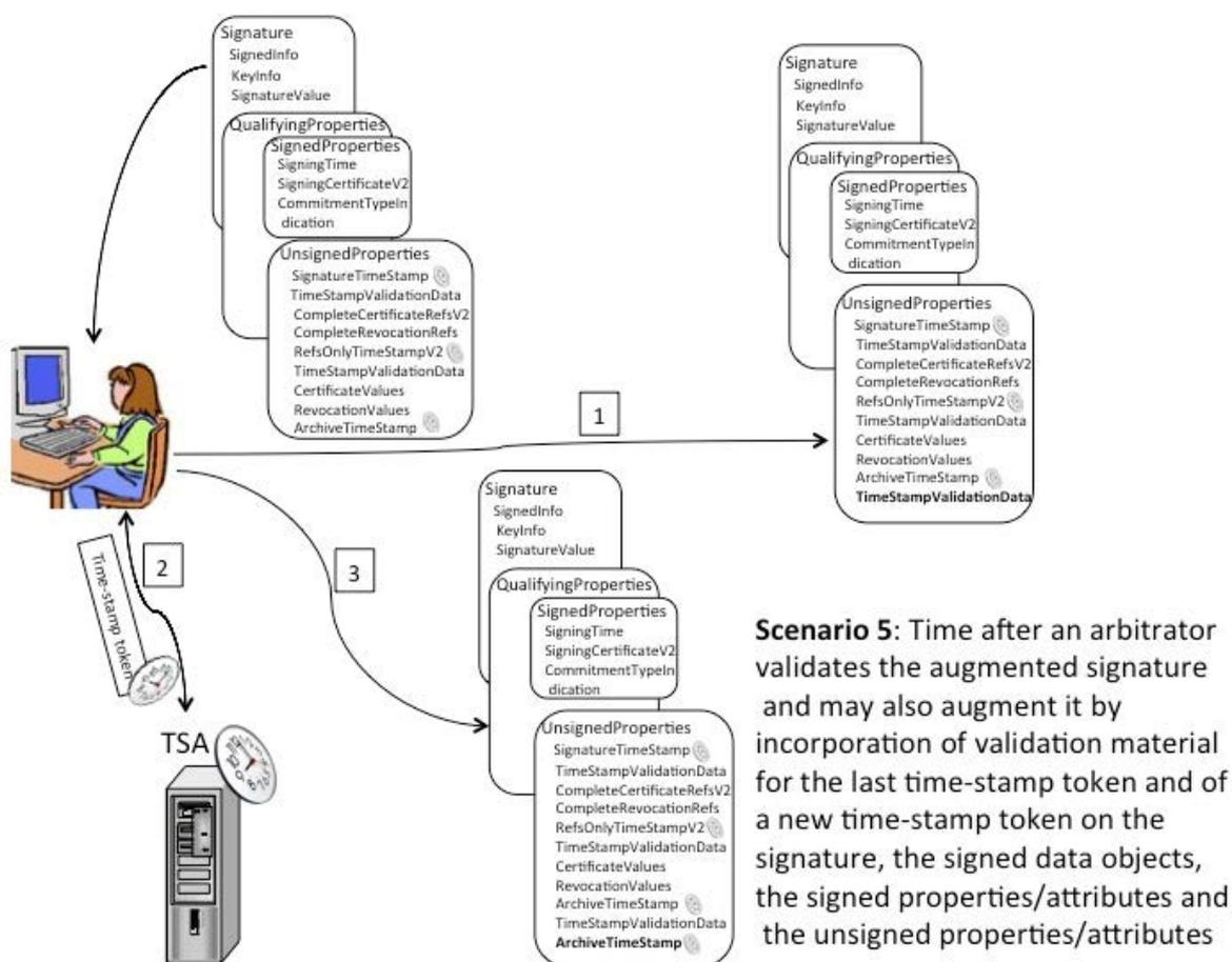
**Figure 6: Arbitrator validating a signature with unsigned properties/attributes, requesting a second archive time-stamp token, and augmenting the signature with the validation material and the archive time-stamp token**
