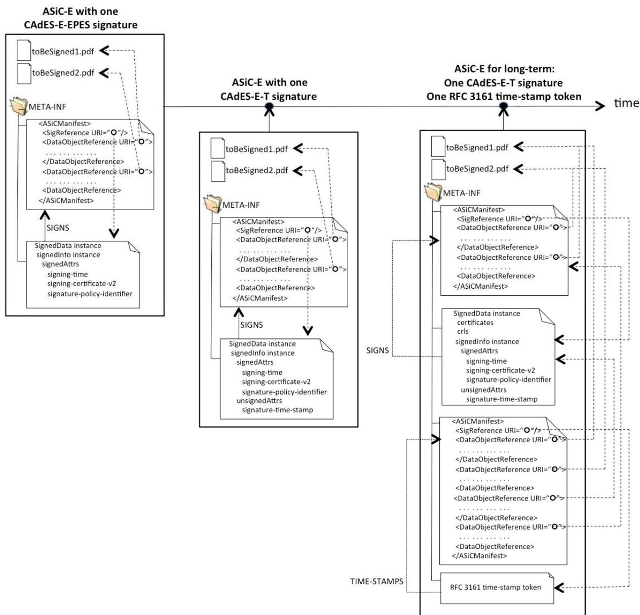
**Figure 17: Transitions for an ASiC-E with one CADES-E-EPES signature up to ASiC-E with availability and integrity of validation material**
