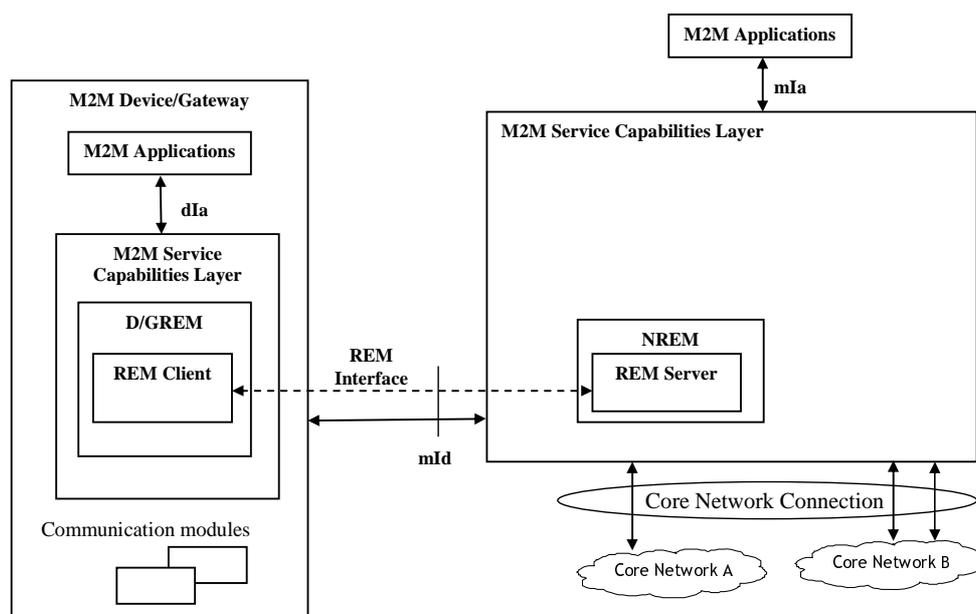
**Figure 8.14: Reference Architecture for managing M2M Device/Gateway**
