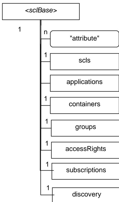
**Figure 8.5: Structure of <scIBase>-resources**
