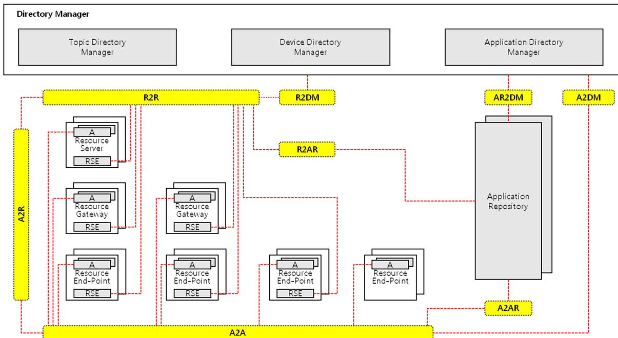
**Figure 10.6: Reference Points of Open M2M Architecture**
