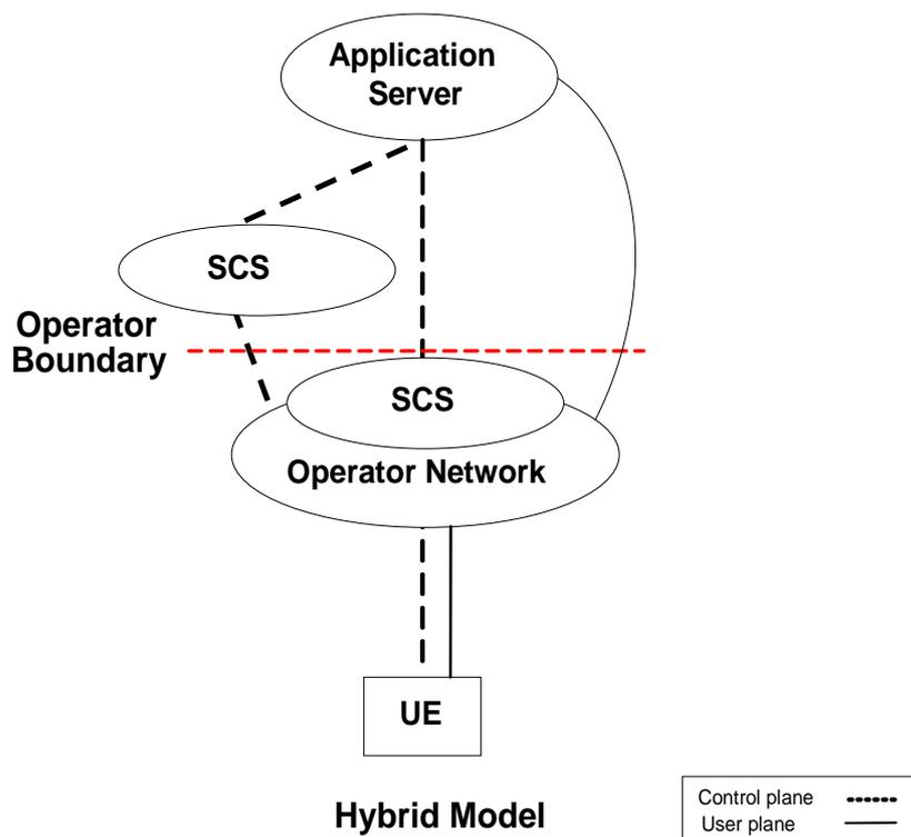
**Figure 12.2: 3GPP Deployment scenarios for hybrid model**
