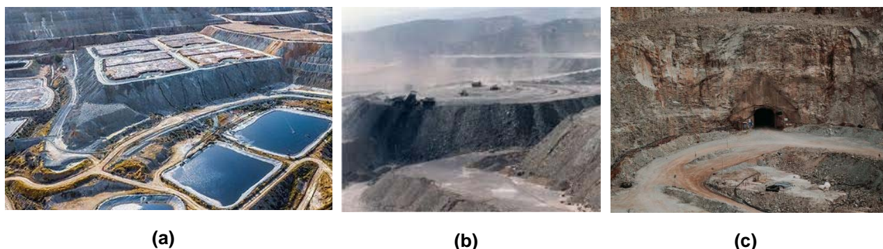
Figure A.5: (a) Leaching pile, (b) Waste dump, (c) Underground mining tunnel portal
