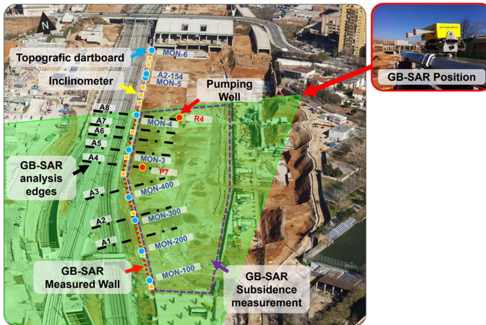
Figure A.3: Examples of GBSAR deployment in a construction site [i.13]
